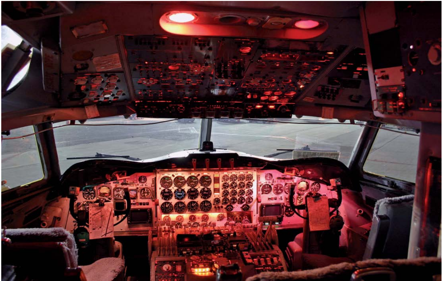
The analogue cockpit of the Electra is a far cry from those found in today's airliners. Of note in this view are the two sets of throttles for pilot and co-pilot. AirTeamImages.com/Daniel Alaerts
