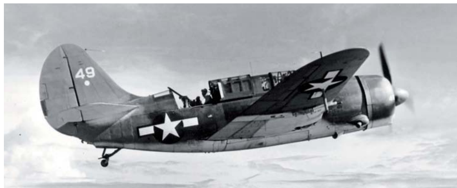
The Helldiver was a chunky aircraft and unlike its Douglas Dauntless predecessor it had an internal bomb bay. US Navy via Robert F Dorr
