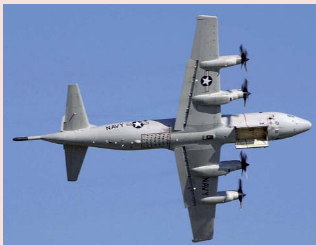
A US Navy P-3C Orion assigned to patrol squadron VP-30 shows off its weapon bay, which can carry a range of anti-submarine munitions, including torpedoes. US Navy/Photographer's Mate 2nd Class Damon J Moritz
