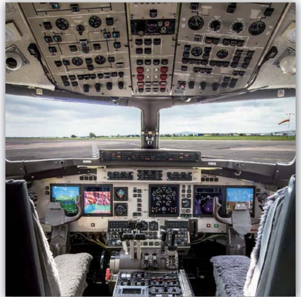
A comparison of the ATP's original cockpit (left), with the upgraded EFIS 'office', gives an idea of the work involved in the refit, as well as the improved operating environment it creates. both West Atlantic
