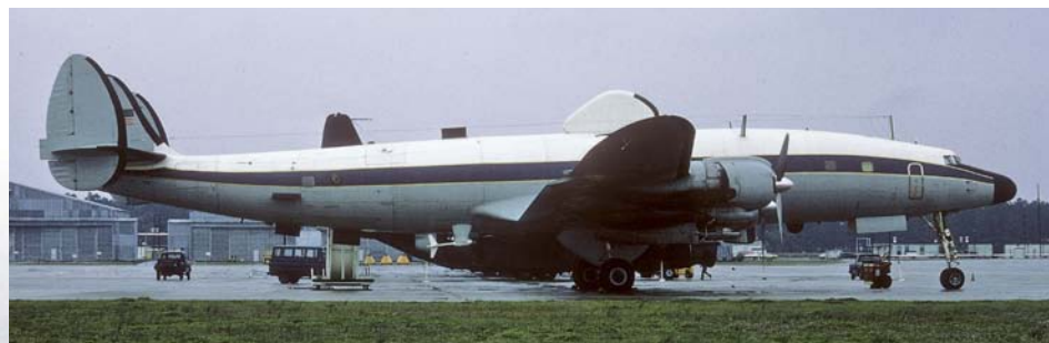
Above: The broadcasting antennas on EC-121S 54-0159 are clearly visible on its upper fuselage, as is the white device lower down just aft of its wing root. Released in flight, the latter stabilised a retractable cable antenna. The aircraft was with the 193rd TEWS, Pennsylvania ANG, at Pope AFB in April 1974. Bob Archer Collection
