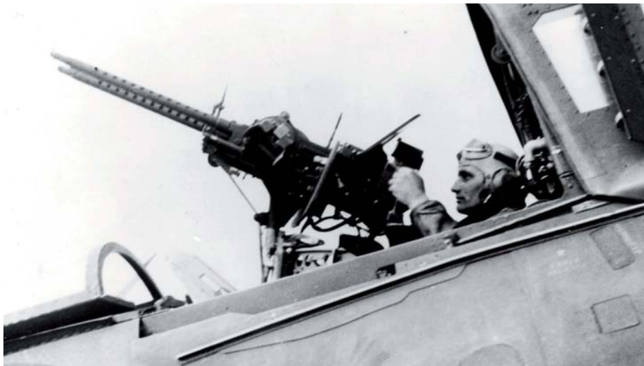
Above: Radioman-gunner Jim Samar sits in the back seat of his SB2C Helldiver with two .30-cal. (7.62mm) flexible machine guns. The rear seat could be rotated to face forward or to the rear. Robert F Dorr Collection
