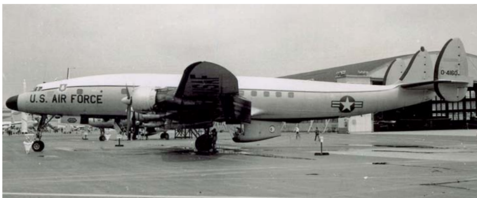
Below: DC-121C 54-0160 with the 4950th Test Wing at Wright-Patterson AFB in around 1970. The gondola mounted on its underside just aft of the wing root housed equipment and an observer. Bob Archer Collection
