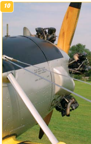
8: Right side of engine cowl showing air intake scoop and engine cylinders. 9: Close up of engine cylinder head (lower right pot). 10: Further detail of the front fuselage and engine cowl showing the wing brace strut and streamlined bracing wires. 11: Close-up detail of access panel on the left side of the engine cowl just behind the engine. 12: The engine cowl left side showing the access panel position and oil filler cap.
