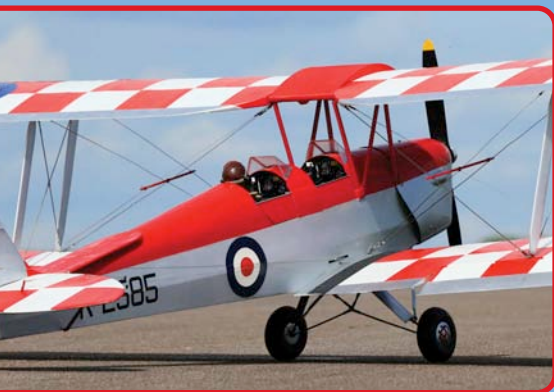
John Thomas's new 1/4 scale Tiger Moth from the venerable Flair kit. NGH 38cc petrol engine, driving a 20"x8" prop.
