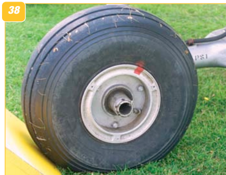
32-38: The main undercarriage in detail - likely to be a major undertaking in the construction of a model of the PT-22. The mechanism features a shock-absorbing arrangement designed to withstand the punishment inevitable when trainee pilots practise landings! With it all 'hanging out', damage could be easily detected and parts quickly replaced.
