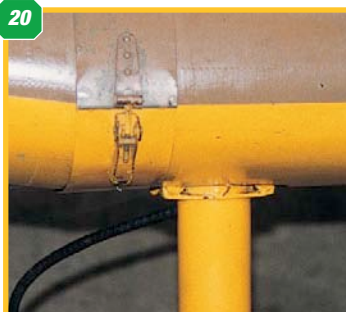
18: Elevator trim tab. 19: Close-up of the tailplane/elevator showing the hinge line and hole through fuselage for the elevator joiner. 20: Panel detail at wing leading edge above the main undercarriage leg. 21 & 22: two views of the main undercarriage leg. Wheel pants were regularly removed at the training establishments. Operating from grass fields, the wheel pants tended to collect mud inside, eventually build-up of which could result in risk of nose-over. 23: The steerable tailwheel unit.
