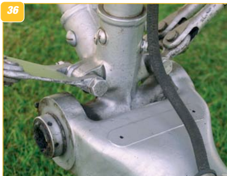
32-38: The main undercarriage in detail - likely to be a major undertaking in the construction of a model of the PT-22. The mechanism features a shock-absorbing arrangement designed to withstand the punishment inevitable when trainee pilots practise landings! With it all 'hanging out', damage could be easily detected and parts quickly replaced.
