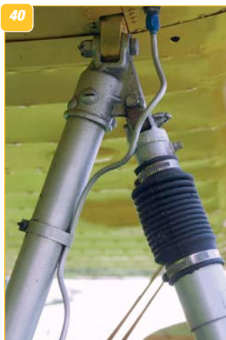
39: The main undercarriage rear anchor point under the wing. 40: Front main undercarriage anchor point on wing undersurface. 41 & 42: Centre-line bubble fairing on fuselage bottom where the main undercarriage bracing wires attach to the fuselage. 43: Pressed metal fairings and access panels on wing underside. 44: The wing root, right hand side, showing rubber panel seals, the cockpit access tread panel and the main bracing strut. 45: Detail of the pressed metal bubble fairing that covers the wing brace anchor point. 46: The cockpit access tread panel on the right hand wing panel. Left side similar. 47: The pitot head on the left wing panel. 48: The right wing, showing the aileron and flap.
