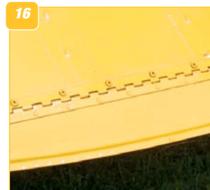
13: The fin and rudder, showing the hinging and the gap between the two vertical surfaces. 14: The tailplane and elevator are similarly hinged and widely separated. 15: Detail of an elevator hinge and anchor point for the bracing wire between the tailplane and the fin. 16: Close-up of the top surface hinge-line of the left side elevator trim tab.
