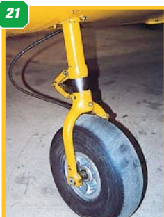
18: Elevator trim tab. 19: Close-up of the tailplane/elevator showing the hinge line and hole through fuselage for the elevator joiner. 20: Panel detail at wing leading edge above the main undercarriage leg. 21 & 22: two views of the main undercarriage leg. Wheel pants were regularly removed at the training establishments. Operating from grass fields, the wheel pants tended to collect mud inside, eventually build-up of which could result in risk of nose-over. 23: The steerable tailwheel unit.
