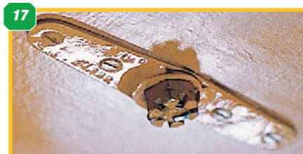
13 & 14: Two views of the tailcone. Note the unshrouded hinge lines and anti-spin strakes. 15: Top surface aileron hinge, reminiscent of typical sport R/C model! 16: Tie-down point on wing underside. 17: Corresponding retainer plate on wing top surface.
