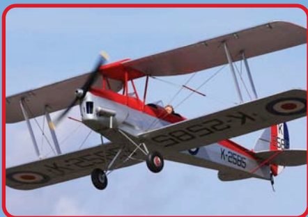
John Thomas's new 1/4 scale Tiger Moth from the venerable Flair kit. NGH 38cc petrol engine, driving a 20"x8" prop.
