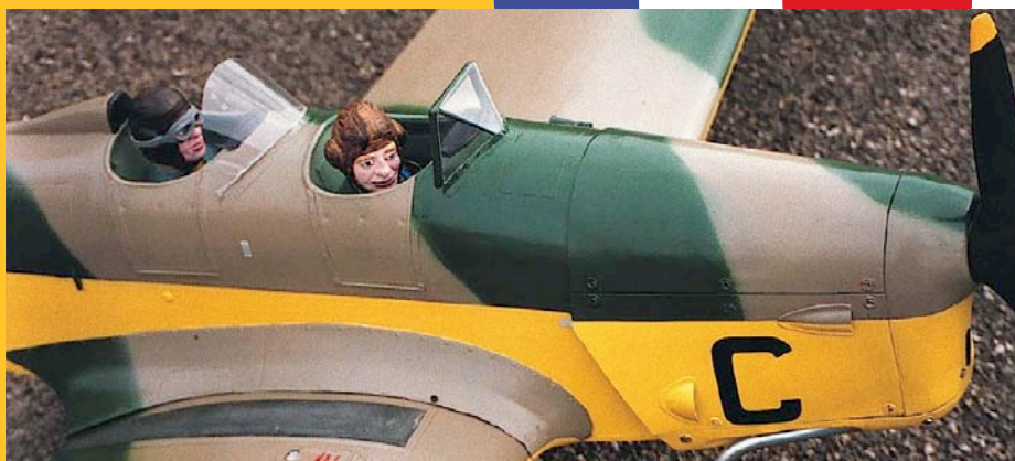
SQUARE-JAW & WHILE KNUCKES! Instructor at the rear and trainee in front. Other details visible here include, wing-tread patch, fuel tank access hatch, air scoops and dummy exhaust pipe.
