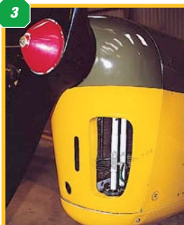
1: The Shuttleworth Collection's machine P6382 at Old Warden is one of the two examples in this photo-detail feature. 2: The line of the engine cowl viewed from across the starboard wing. 3: The nose, showing the panel lines and air intake. Note the size of the panel fasteners. 4: A further view of the cowl from the starboard side. 5: Head-on view of the nose showing the exhaust exit.
