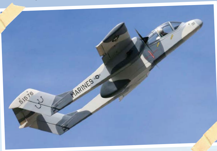
David Osborne's 1/5th scale electric Bronco. Twin Axi 2328 out-runners, driving 17"x12" props.
