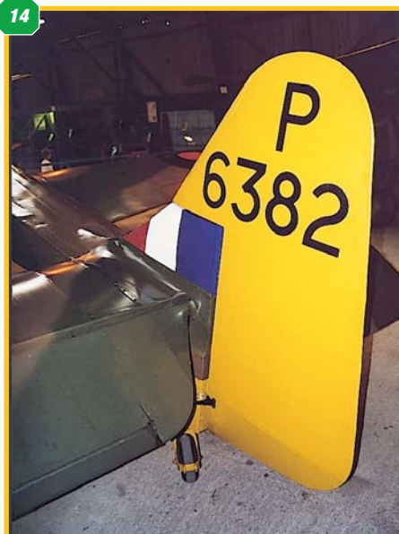
13 & 14: Two views of the tailcone. Note the unshrouded hinge lines and anti-spin strakes. 15: Top surface aileron hinge, reminiscent of typical sport R/C model! 16: Tie-down point on wing underside. 17: Corresponding retainer plate on wing top surface.
