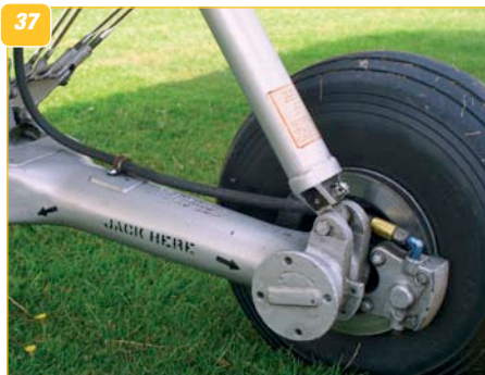
32-38: The main undercarriage in detail - likely to be a major undertaking in the construction of a model of the PT-22. The mechanism features a shock-absorbing arrangement designed to withstand the punishment inevitable when trainee pilots practise landings! With it all 'hanging out', damage could be easily detected and parts quickly replaced.
