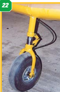
18: Elevator trim tab. 19: Close-up of the tailplane/elevator showing the hinge line and hole through fuselage for the elevator joiner. 20: Panel detail at wing leading edge above the main undercarriage leg. 21 & 22: two views of the main undercarriage leg. Wheel pants were regularly removed at the training establishments. Operating from grass fields, the wheel pants tended to collect mud inside, eventually build-up of which could result in risk of nose-over. 23: The steerable tailwheel unit.
