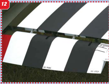
11: Supplied wing panels have all the scale surface details moulded in. 12: Fowler type flaps drooped for the camera. Note flap-degree verniers. 13: Four .50 calibre cannon per wing. 14: Crisp control surface hinge details throughout the model.
