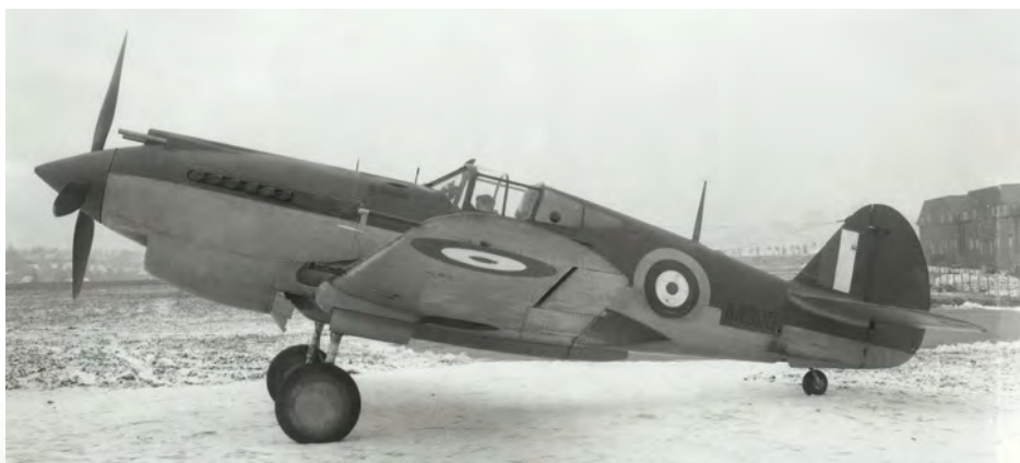
Above: Parked in the snow at Yeovil, this Curtiss fighter (AX900) underwent Westland's 'anglicisation' with different controls and Imperial instrumentation introduced to examples originally destined for France. The type later served with the RAF in large numbers as the Tomahawk.
