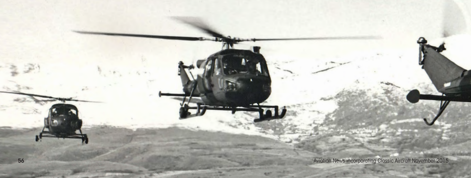
Below: The Westland Scout (army) and Wasp (navy) helicopters were developed from the Saunders-Roe P.531 programme, which Westland took over in 1959. These three Scout AH.1s were operated by Britain's Army Air Corps.
