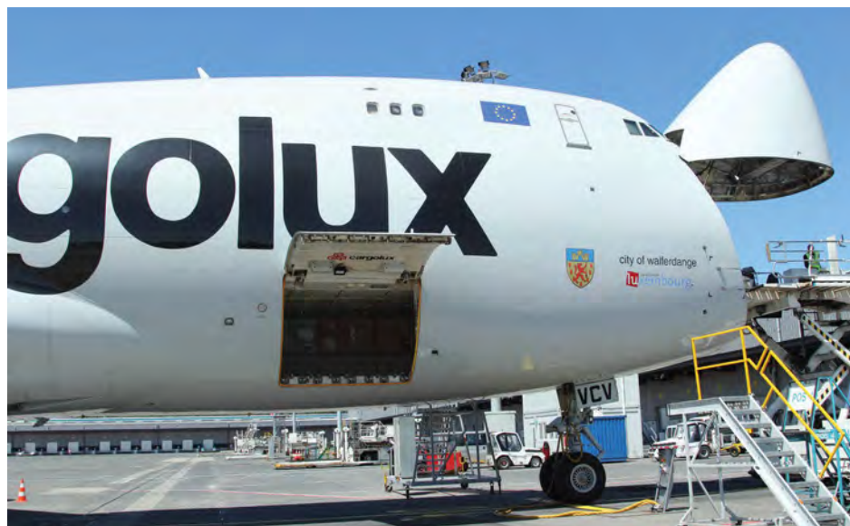
Above: Cargolux's 747s have two cargo holds, one each in the belly and on the main deck. Key-James Ronayne
