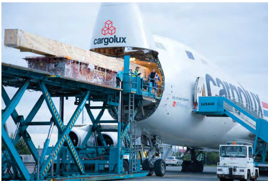
Outsized cargo is one of the areas Cargolux specialises in. One of the benefits of Boeing 747 freighters is the nose cargo door, which makes loading long objects easier. Cargolux
