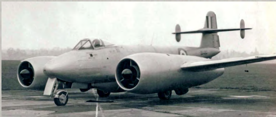
Above: After switching its focus to helicopter production, Westland made an unusual foray back into aircraft matters, modifying Meteor F.4 RA490 for the Royal Aircraft Establishment at Farnborough for jet deflection tests. The large outlet for the deflected thrust can be seen below the port engine nacelle. The aircraft first flew in this configuration in early 1954.
