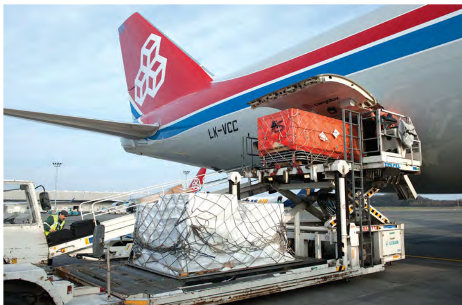
Above: Cargolux's 747s have two cargo holds, one each in the belly and on the main deck. Key-James Ronayne
