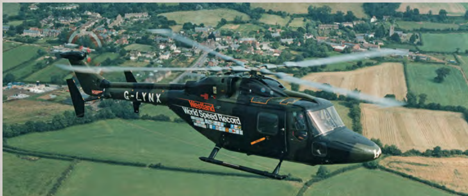
Above: Westland's Lynx demonstrator G-LYNX became the most famous helicopter in the world when, in August 1986, piloted by Trevor Egginton, it set an absolute world speed record for helicopters by achieving 400.87km/h (249.09mph).
