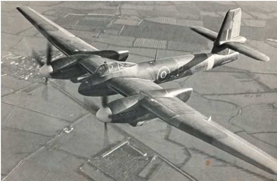
Above: Despite not seeing frontline service, the Welkin high-altitude fighter project was important to Westland's future in establishing the company as a world leader in pressurisation and oxygen equipment for high-altitude flight.
