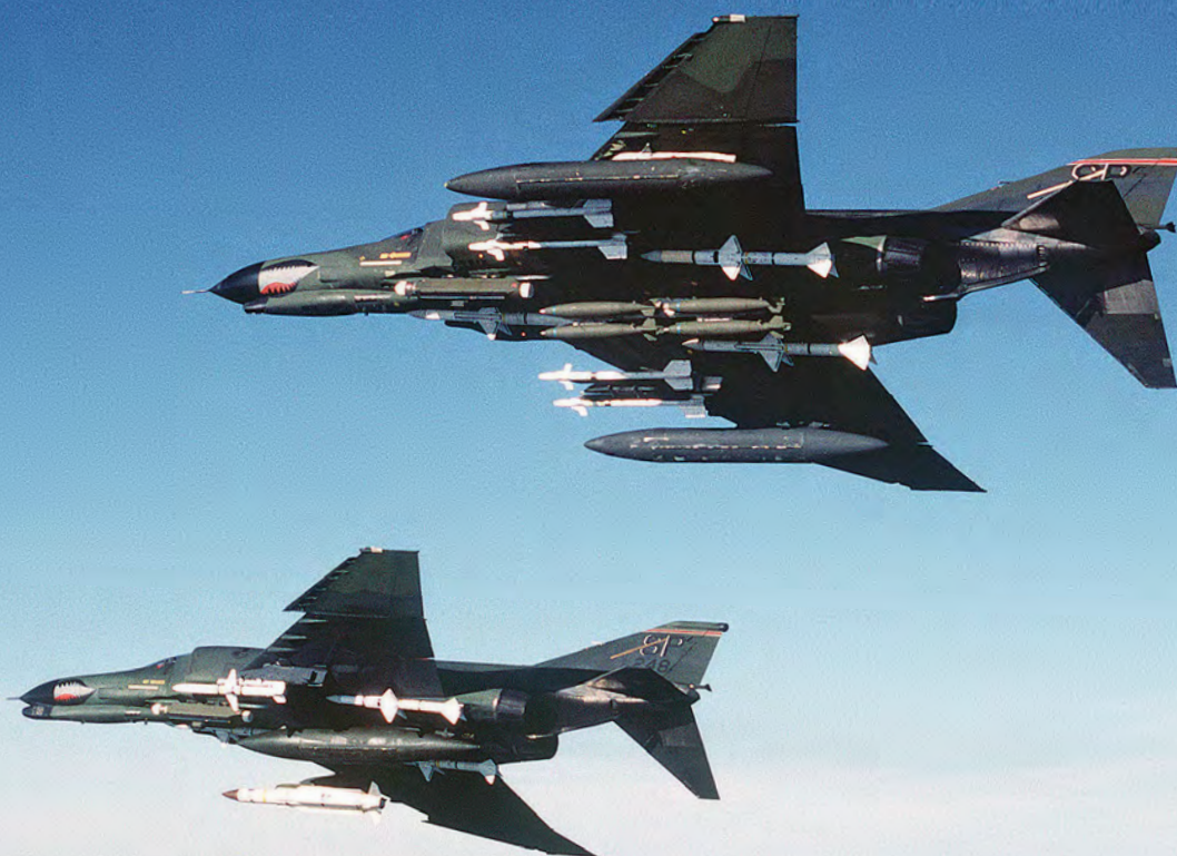
Above: Three shark-mouthed Phantoms of the 480th TFS/52nd TFW. Two F-4Es flank an F-4G Wild Weasel. The aircraft are armed with an AGM-78 Standard Anti-Radiation Missile (F-4G), AGM-45 Shrike air-to-surface missiles, AIM-7 Sparrow III and AIM-9 Sidewinder air-to-air missiles. The aircraft are equipped with electronic countermeasures pods. The F-4E in the foreground is also carrying four Mk82 general purpose bombs. USAF National Archives
