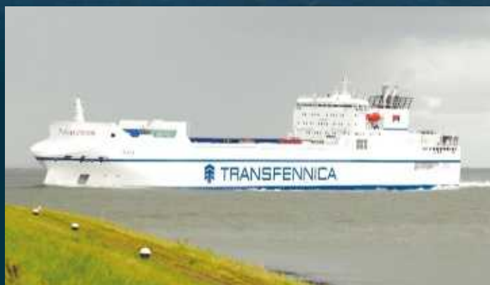
ABOVE The ro-ro cargo ship Plyca (28,289gt) was the first of Transfennica's six container ro-ros to be fitted with scrubbers, by widening the funnel. She is seen heading past Terneuzen, on the river Scheldt, having sailed from Antwerp.
