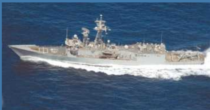
ABOVE Aerial view of USS Steven W. Groves. Note the Mk.13 missile launcher forward of the bridge is missing and there is a cap in its place
