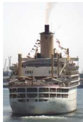
ABOVE Orsova departing Southampton on a cruise. Note the high bridge wings. Like her sisterships Oronsay and Orcades, and the later Oriana, she had her navigating bridge high amidships at the centre of rotation, unique to large passenger liners.
