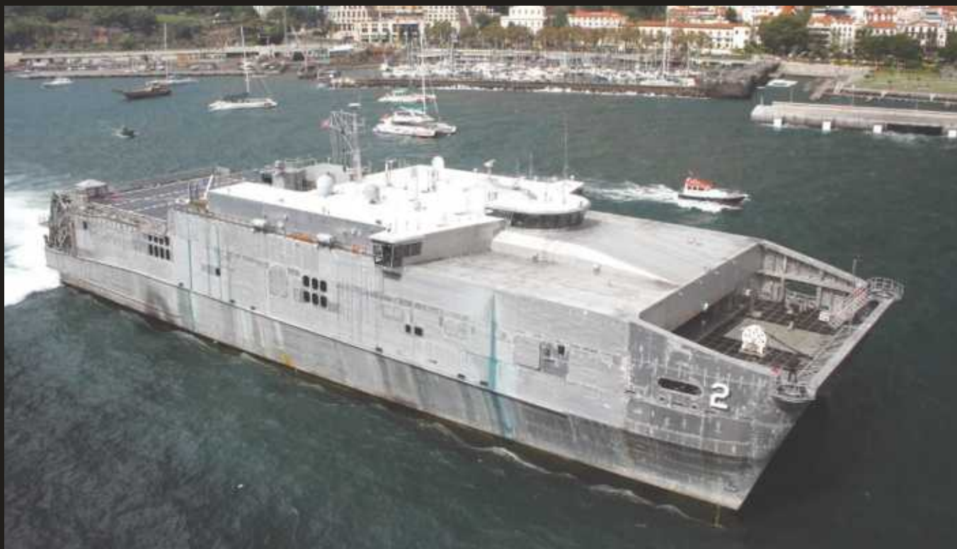
▲ The Austral-built Spearhead class Joint High Speed Vessel USNS Chockaw County departing Madeira on 15 October 2015 and heading into very rough seas. She has a flight deck for helicopter operations and a loading ramp that allows vehicles to drive quickly on and off. PAUL DALLOWAY
