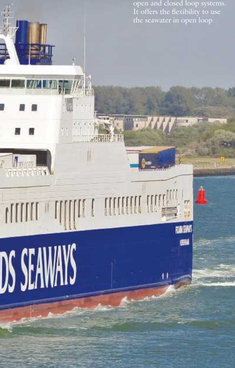
ABOVE Clearly showing the widened funnel, which incorporates the scrubber, Containership VI heads for Rotterdam on the service from the Baltic.
