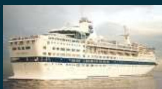
1991 • New look as RCCL's Viking Serenade, with car decks converted to extra cabins.
