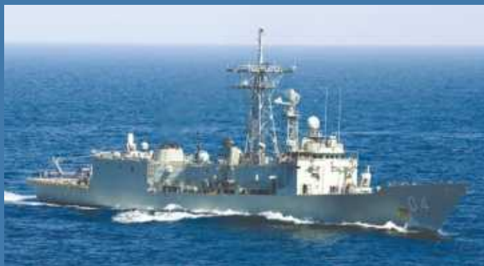
ABOVE Designed as anti-submarine warfare frigates the Perrys, such as USS Aubrey Fitch, were fitted with torpedo tubes and dedicated ASW helicopters.
