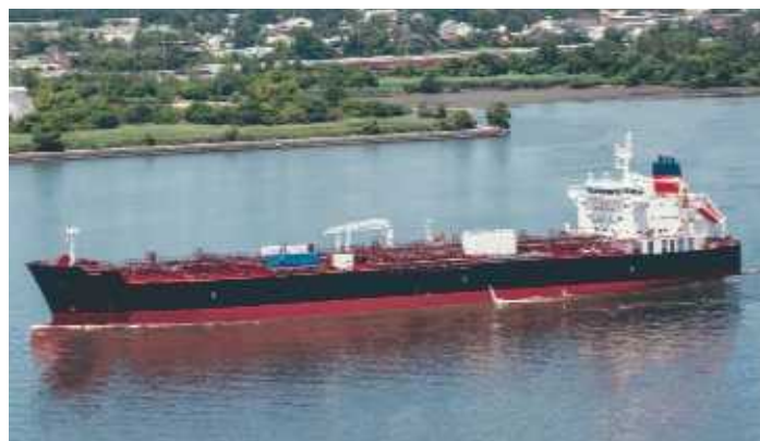
ABOVE The 600ft-long tanker Ohio is the first of four newly built, LNG-ready product tankers for the US coastwise trade and can carry crude oil or refined petroleum products. CROWLEY
