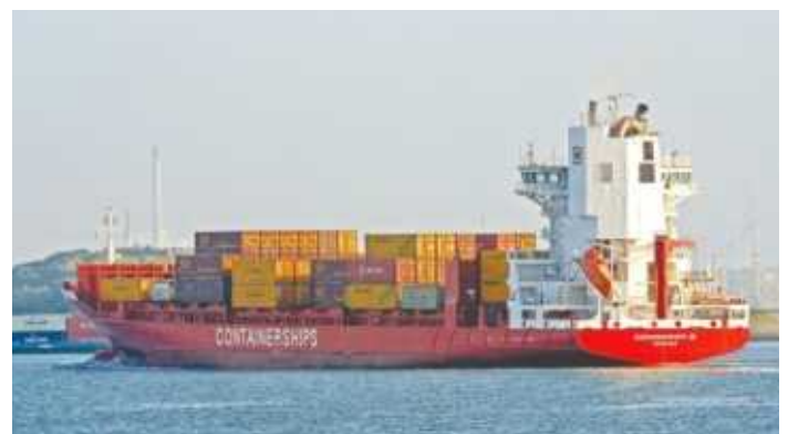
ABOVE Clearly showing the widened funnel, which incorporates the scrubber, Containership VI heads for Rotterdam on the service from the Baltic.
