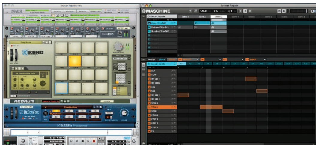
FIG. 1: Maschine Groups are set up to step-sequence Reason Kong, Redrum, and Dr.OctoRex modules via Advanced MIDI routing in Reason's Hardware Interface.
