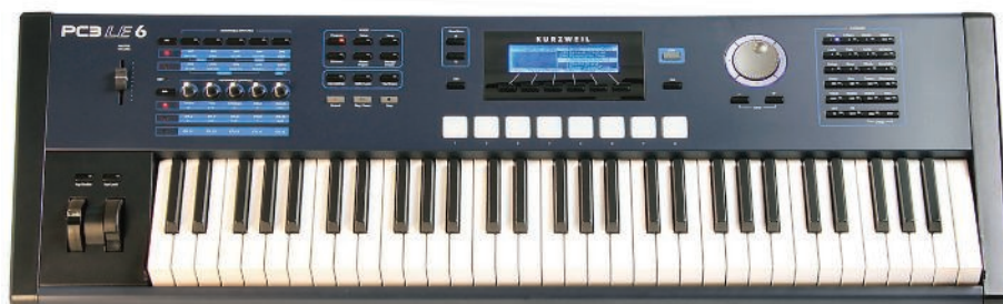
FIG. 3: PC3LE's user controls include a 24-button bank of category controls, eight drum pads, and five user-configurable control knobs.
