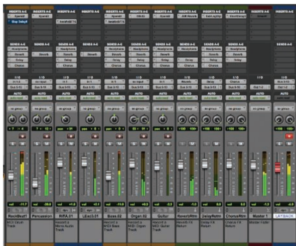
FIG. 5: I've routed all of the track outputs to Bus 9-10 and matched the input for the destination track.
