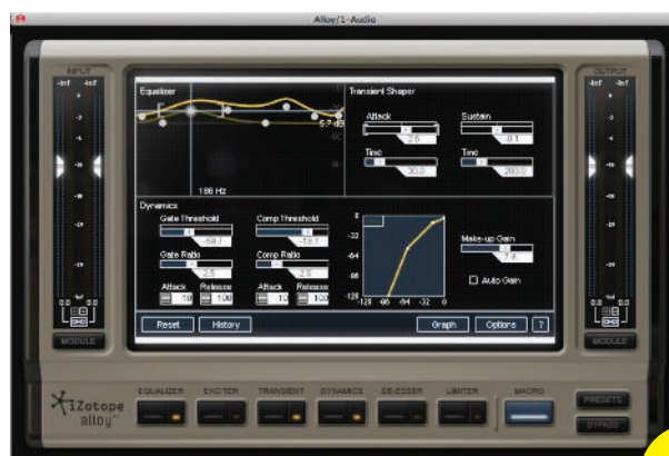
FIG. 1: Alloy's Macro page provides live-editable access to all of the main elements of a Macro Preset from a single page, and can be customized to create your perfect mixing experience.
