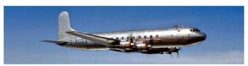
Above: The Tudor 7, G-AGRX, was an attempt to rectify the type's performance shortfalls by replacing the Rolls-Royce Merlins with Bristol Hercules engines. Unfortunately, the re-engining delivered little improvement. Avro Heritage
