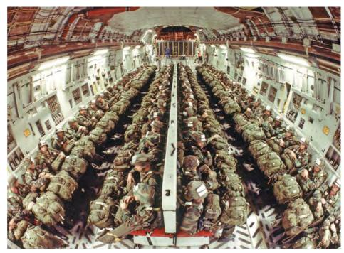
A C-17A's cabin can carry 102 paratroopers using 54 permanently installed sidewall seats and additional seating in the centre. Boeing
