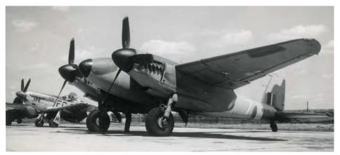
Three hundred FB.26s were built in Canada and were essentially FB Mk.VIs but with Packard Merlin engines. Key Collection
