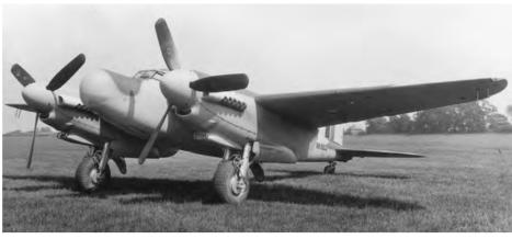
The Mosquito NF Mk.XXX had two-stage superchargers for improved altitude performance and can be distinguished by the lip intakes immediately behind the spinners. Aircraft RK953 was fitted with the US-built Al Mk X radar as well as the Serrate device that tracked the Lichtenstein radar used by German night-fighters. Key Collection
