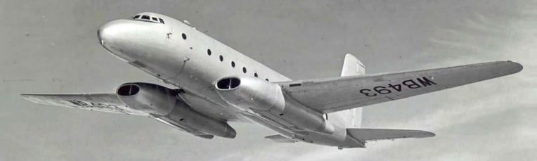
Avro Ashton WB493 was one of the six redundant Tudor 2 airframes rebuilt for research purposes with nosewheel undercarriages and Rolls-Royce Nenes. This machine was later fitted with Bristol Olympus engines in outboard nacelles. BAE Systems
