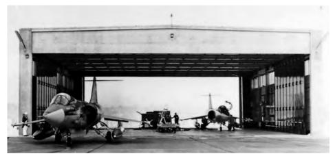
An alert scramble of two air defence F-104Gs of JG 71 *Richthofen* at Wittmund. The aircraft are configured with two underwing tanks, AIM-9 Sidewinder air-to-air missiles on wingtips rails and armour piercing and high explosive rounds for the internal M61 cannon. Wilhelm Göbel
