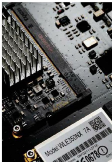
Inside the Altair: note the Complex WiFi adapter in the foreground.
