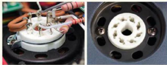
PrimaLuna tube socket. Left: Bottom view, showing point to point wiring. Right: top view, showing socket bolted to panel.
