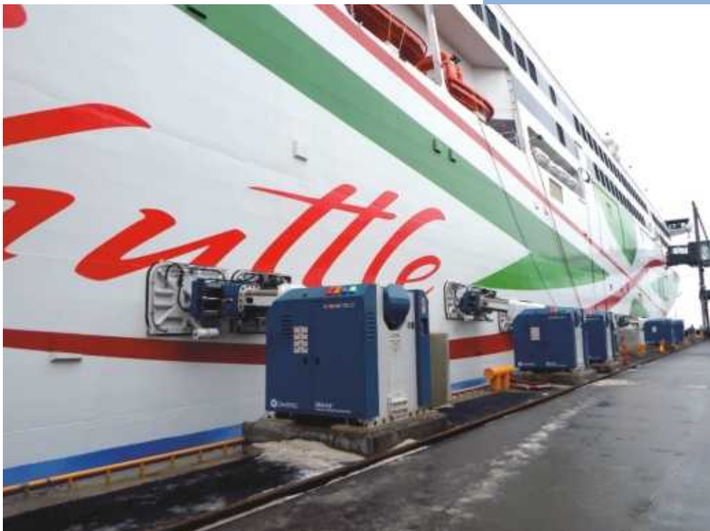
▲ Megastar docked in Helsinki, where the captain berths the ship at West Harbour's new Terminal 2 using the automatic mooring system's vacuum pads.
