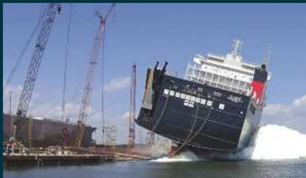
▲ The new con-ro ship El Coquí is launched at Pascagoula in March. As well as standard containers, she can take up to 300 reefers. COMPANY PHOTO
