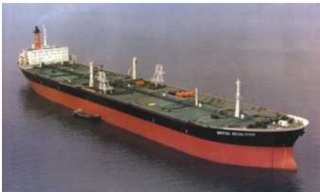
▲ The 1974-built VLCC British Resolution was built by Mitsubishi in Nagasaki and delivered on 8 November 1974. Powered by steam turbines, she had a deadweight tonnage of 270,665 and could carry 160,000 tons of oil. She was scrapped in 1999 at Alang, India.
