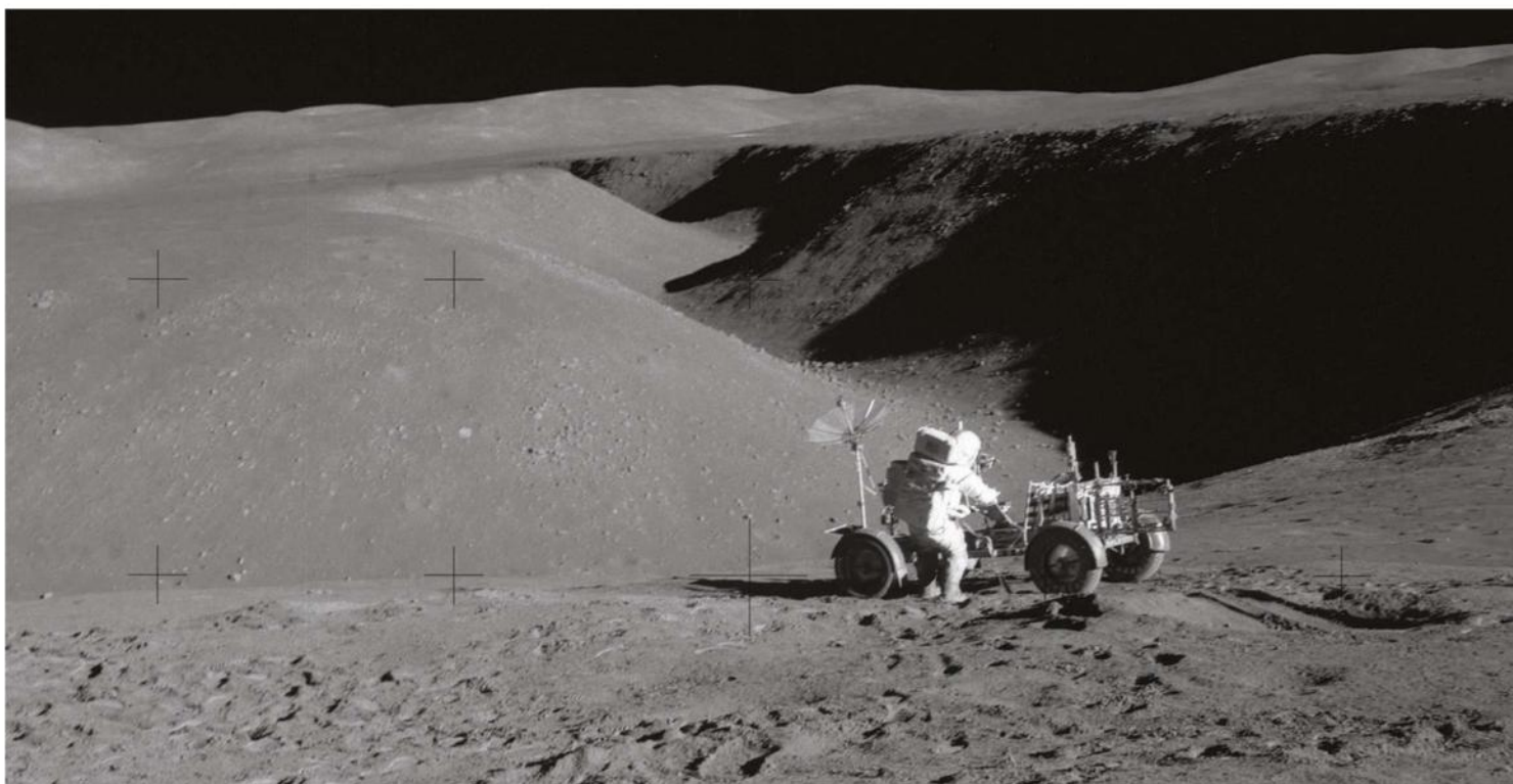
◀ Astronaut David Scott drives the lunar rover during Apollo 15. The battery-powered buggy had to be unfolded before it could be used
