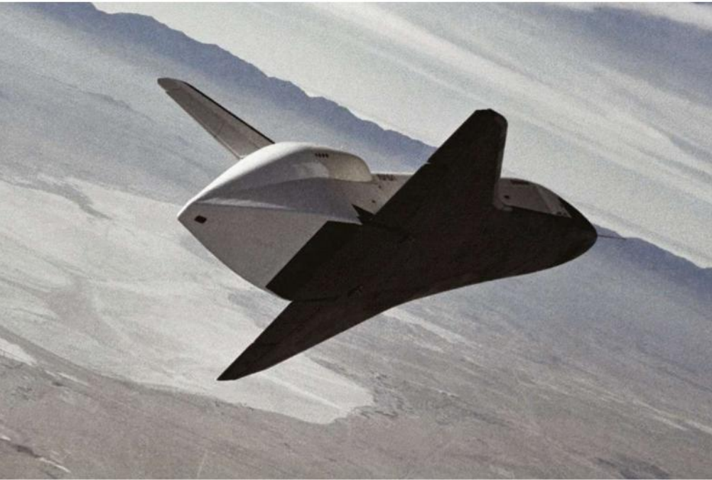
▲ The prototype Space Shuttle Enterprise flies over Rogers Dry Lake, California, in September 1977 to test the Shuttle's ability to glide in for a landing. These approach and landing tests lasted nine months
