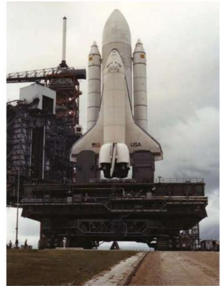
▲ Enterprise rolls out to the launch pad on 1 May 1979. A test machine, it had no engine or heat shield and never flew into space
