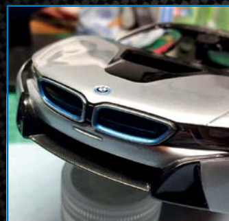
You can get a great gloss black finish using Zero paints Semi Gloss Black, finishing it with the company's two-part 'Diamond Finish' clear varnish
