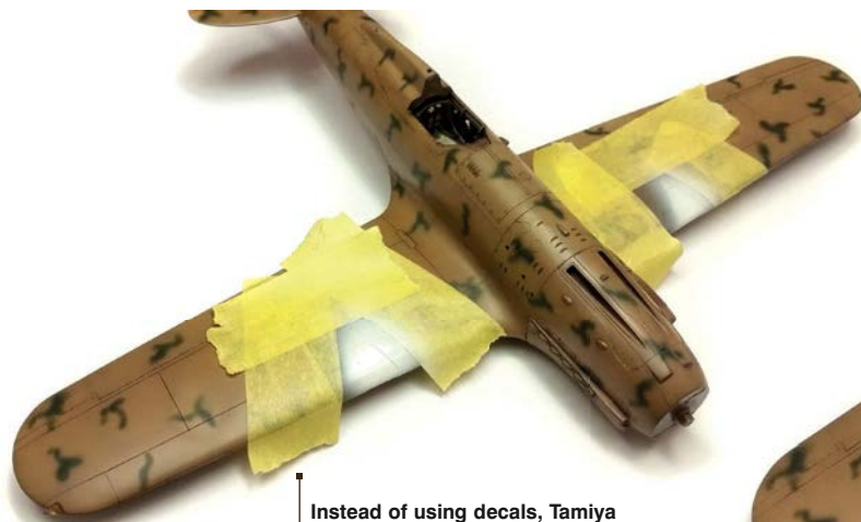
Instead of using decals, Tamiya masking tape was used to blank off the overspray areas
