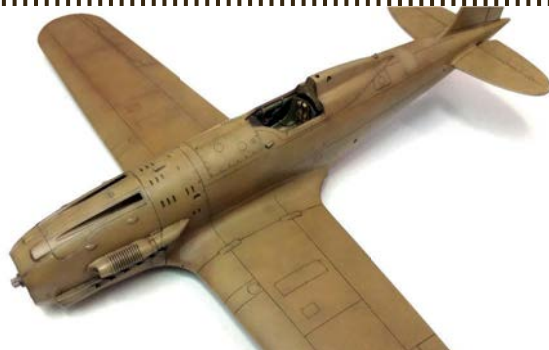
With the brown oil paint wiped off, an overall staining effect is created, leaving the panel lines darkened
