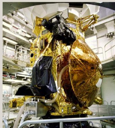
The Cassini spacecraft, including the Huygens probe destined to punch through Titan's atmosphere to touch down on its surface, sits awaiting launch atop a Titan ICBV rocket in 1997. During launch, a payload fairing, or nose cone, protected the craft. NASA
