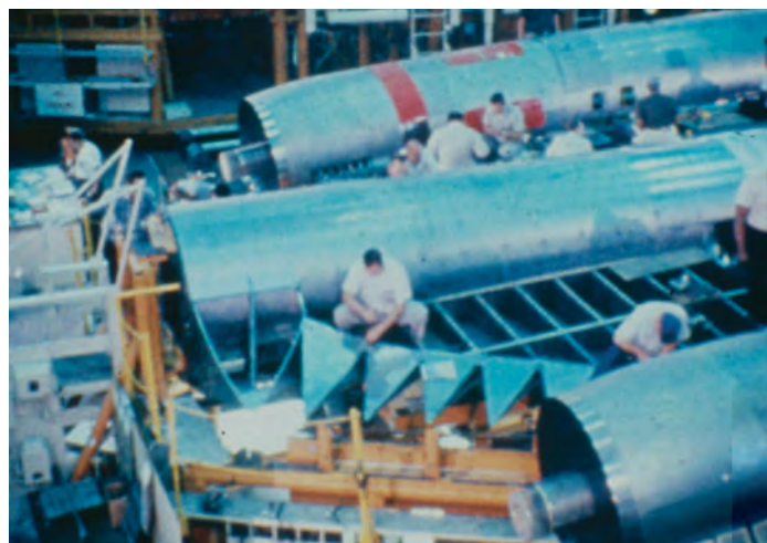
Above right: A frame grab of an A-12 being constructed which shows the serrated titanium wing leading edges before the high-temperature-resistant triangular shaped RAM was installed. Lockheed Martin
