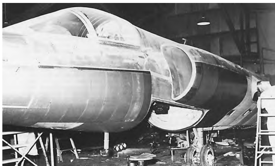
Above left: A U-2 having radar-absorbent material (RAM) – Echosorb – applied to its lower fuselage. Lockheed Martin
