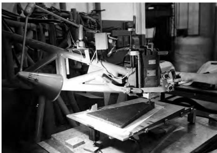
Above left: A monocoque wing fillet of RAM undergoing construction. Lockheed Martin
