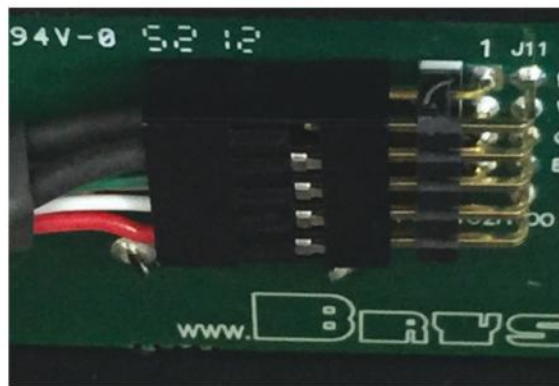
Clockwise from top: BDP-3 internal components; front panel data cable connected upside down (red cables at bottom rather than on top); Bryston USB WiFi Adapter/Dongle.
