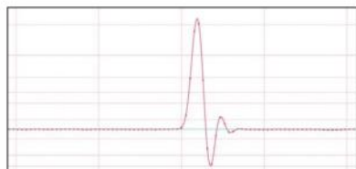
Fig.6 Mytek Brooklyn DAC with MQA enabled, non-MQA impulse response (one sample at 0dBFS, 96kHz sampling, 100μs/horizontal div.).
