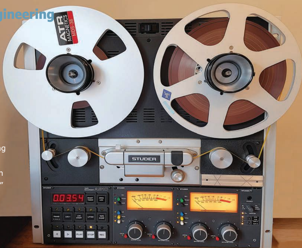
Photo 1: Professional 1/4" stereo recorders, such as the Studer A810 shown here, usually record on two tracks and in one direction only.
