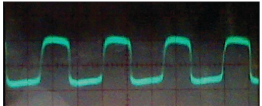
Figure 3: This waveform was produced by the circuit of Figure 2 when limiting.
