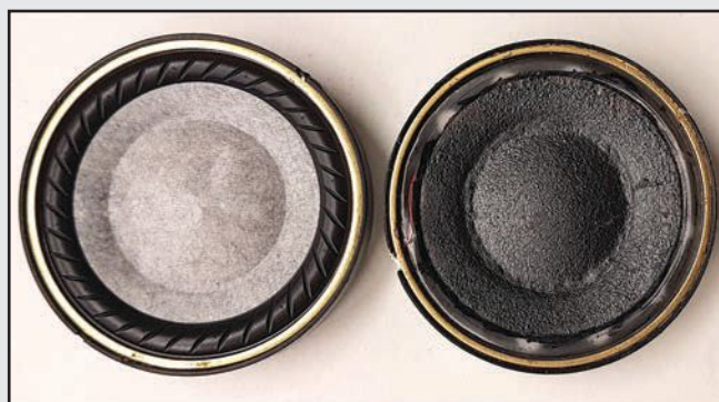
The 40 mm cellulose headphone driver (left) and a prototype 40 mm GrapheneQ headphone driver (right).
