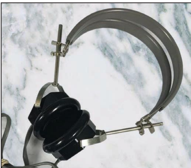
Photo 2: Headsets like these (using either crystal or telephone-quality magnetic elements) were often the sound operator's only way of getting an idea of the sound in a venue in the 1950s.
