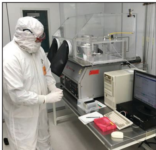
GraphAudio staff uses this Chemical Vapor Deposition (CVD) tool for Graphene development.
