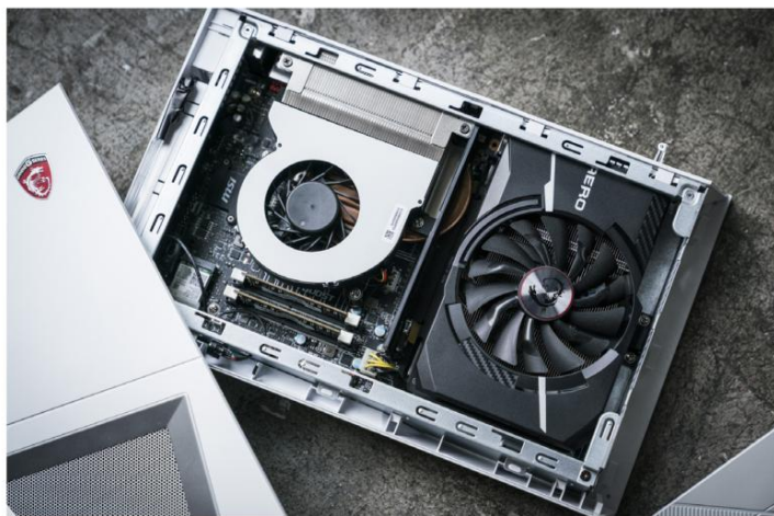
RAM and CPU on the left, GPU on the right.
