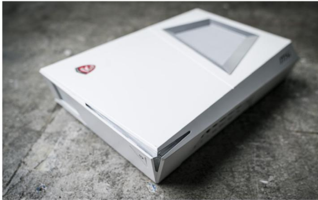
It's not illuminated here, but that odd "Y" shape on the corner is the RGB LED zone.
