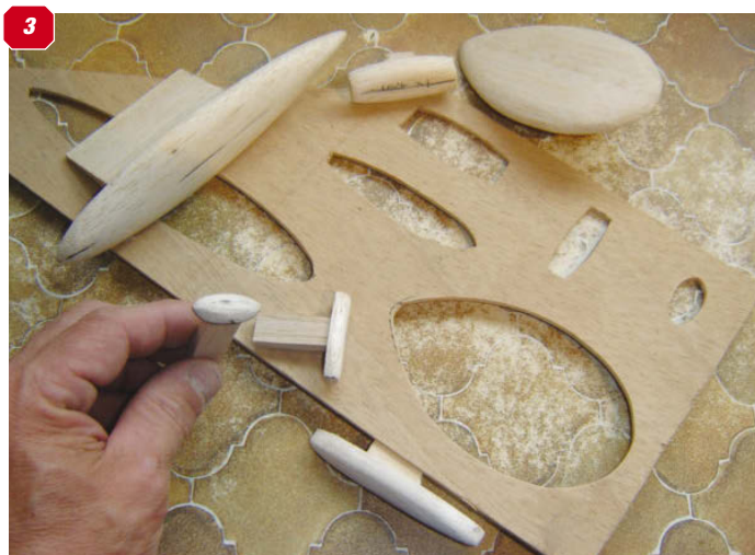
1 & 2: The shape of each part to be moulded is transferred from the plan onto sheet and block balsa as required. 3: Having cut out and shaped the plugs, a handle is glued on each one after drawing round them to create the draw plate from ply. The holes are cut out approximately 1mm oversize. 4: Here we have the plug for the cannon blister on top of the wing held in a small bench vice ready for moulding. 5: The first mould taken from this plug. I found that if too thin material was used, I would end up with a very flimsy moulding that would not be strong enough. 30-thou. sheet is about right for this size of component. 6: This is the heatgun used, and I attached the acrylic to the ply former with bulldog clips which get very hot when heated (guess how I found this out!).
