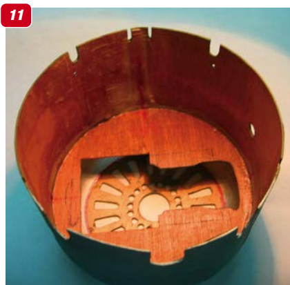
11: Engine cowl interior, showing the cooling baffle referred to in text; the front part of the cowl started life as a kitchen wok. 12: The finished cowl showing the fretted shroud at the front. The metal front end of the cowl was fashioned from a metal Wok, while the cylindrical rear is made of 1/64" ply, wound around cardboard formers. 13: The main undercarriage complete and in a state ready to fit the the bottom of the fuselage.
