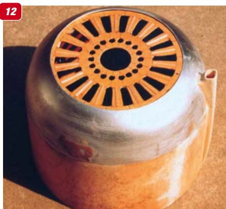
11: Engine cowl interior, showing the cooling baffle referred to in text; the front part of the cowl started life as a kitchen wok. 12: The finished cowl showing the fretted shroud at the front. The metal front end of the cowl was fashioned from a metal Wok, while the cylindrical rear is made of 1/64" ply, wound around cardboard formers. 13: The main undercarriage complete and in a state ready to fit the the bottom of the fuselage.
