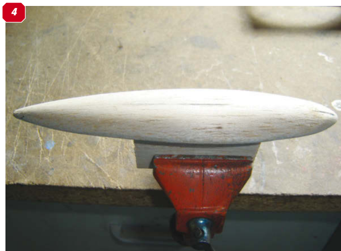
1 & 2: The shape of each part to be moulded is transferred from the plan onto sheet and block balsa as required. 3: Having cut out and shaped the plugs, a handle is glued on each one after drawing round them to create the draw plate from ply. The holes are cut out approximately 1mm oversize. 4: Here we have the plug for the cannon blister on top of the wing held in a small bench vice ready for moulding. 5: The first mould taken from this plug. I found that if too thin material was used, I would end up with a very flimsy moulding that would not be strong enough. 30-thou. sheet is about right for this size of component. 6: This is the heatgun used, and I attached the acrylic to the ply former with bulldog clips which get very hot when heated (guess how I found this out!).
