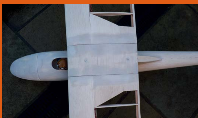
Inset bolts on the Wolf's centre section
