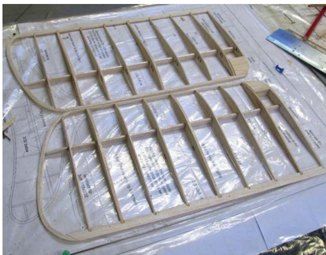
Okay, so there's a spar missing in the wings but at least you can see pretty much how they go together, while the fuselage lurks in the background.
