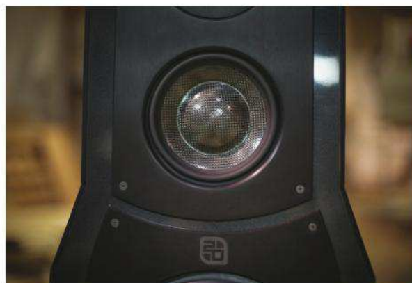
Clockwise from left: The Viginti's back-panel plaque; among the elements that comprise the Viginti's internal labyrinth is the bass-clef-like shape in the foreground; one of the Viginti's carbon-dome midrange drivers.
