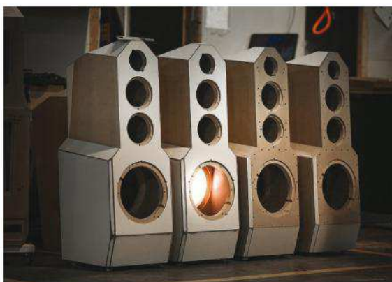
The earlier Andra models didn't have an MTM upper-frequency array and used a single large woofer.
