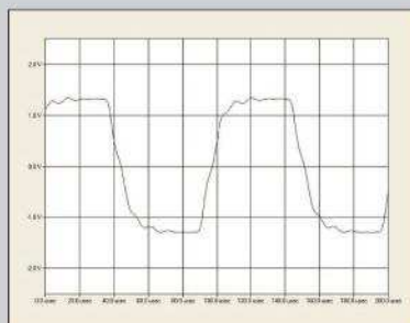
Fig.3 Rogers 65V-1, EL34s, Ultralinear mode, small-signal, 10kHz squarewave into 8 ohms.
