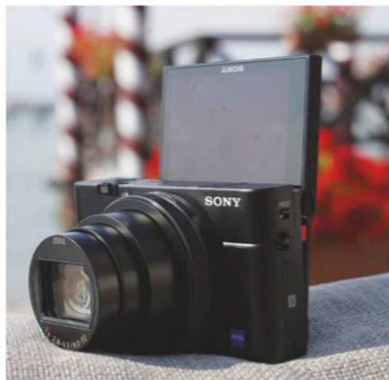
The LCD tilts upwards 180 degrees for selfies or vlogging
