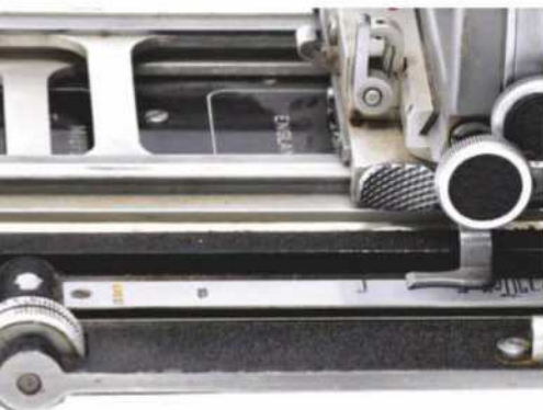
The focusing scale on the side of the bed
