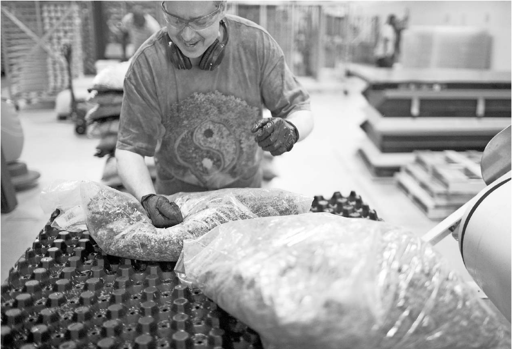
Above, preparing mycelium fungus, which forms the roots of mushrooms as they grow in places like compost piles, at Ecovative's factory. Below, its packaging using mycelium.
