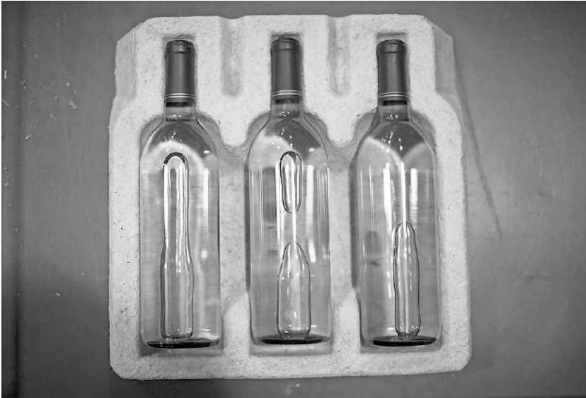
Above, preparing mycelium fungus, which forms the roots of mushrooms as they grow in places like compost piles, at Ecovative's factory. Below, its packaging using mycelium.
