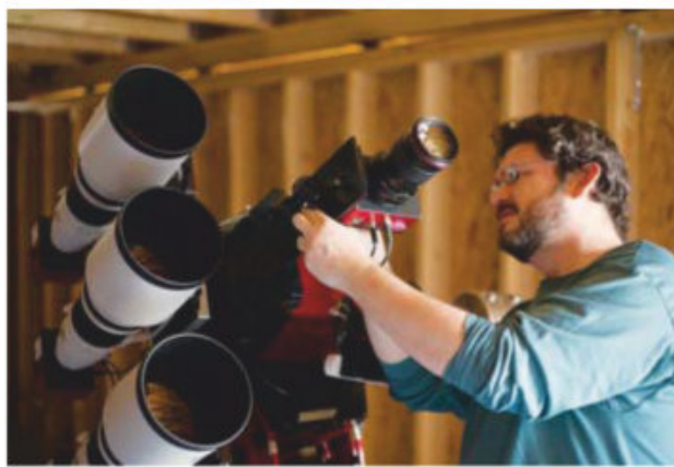
▲ TRIPLED GAZE Roberto Abraham mounts an autoguider camera on the proof-of-concept three-lens prototype.
