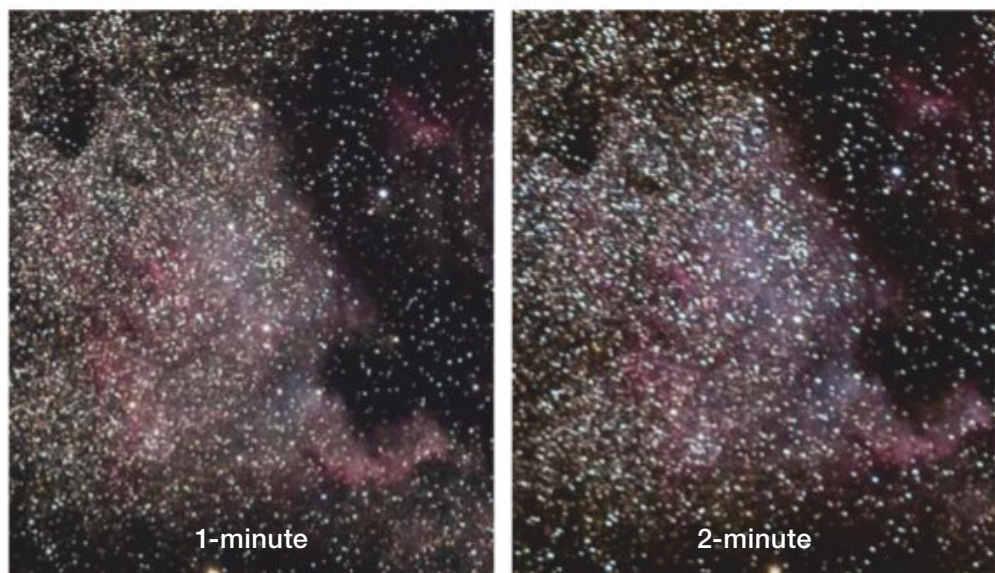
◀ When using a 135-mm telephoto lens, most 1-minute exposures (at left) were only slightly trailed. But every 2-minute exposure (at right) showed some level of trailing, in keeping with the Mini Track’s exposure limit engraved on its sector gear.
