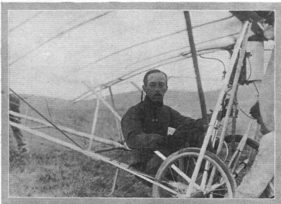
In the above central view of the "Demoiselle" M. Santos Dumont is occupying the somewhat rough and ready canvas seat that is provided for the pilot. He has in his right hand the elevating lever, which moves the universally-jointed tail up or down; his left hand is grasping the small wheel which serves to steer the machine by moving the rudder sideways, and at his back is the lever that enables him to flex the wings by leaning his body over to one side or the other.
