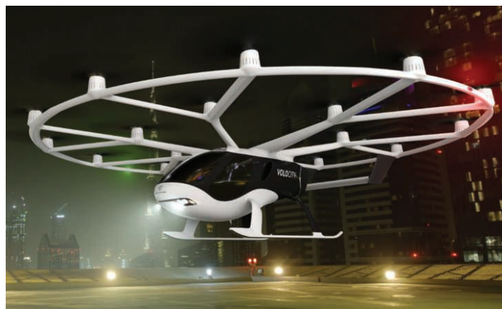
Designed to seat two people, the aircraft will have a range of 19nm
