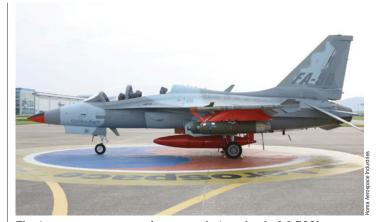
The type can carry a maximum combat payload of 4,500kg
