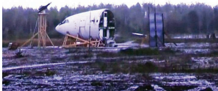
Missile maker Almaz-Antey tested the effects of a Buk explosion
