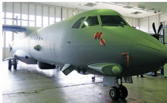
Alterations have increased the fuselage length by around 1.5m
