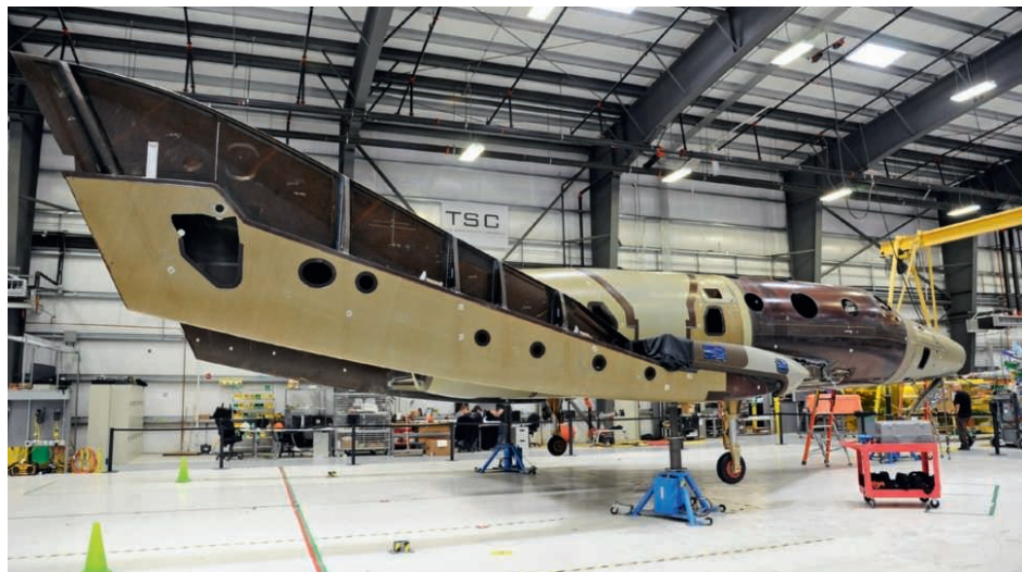
Virgin Galactic’s SS2-2 in construction; subtle changes reflect accident report findings
