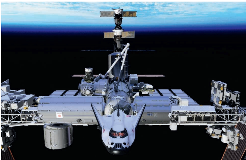
Reusable spaceplane could resupply the International Space Station, and act as temporary module
