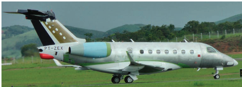
The Legacy 500 has completed taxi runs, where the aircraft was taken to a speed of 80kt
