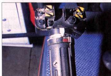
(Top) the compact instrument panel offers good visibility; (above) the twist-grip throttle is made largely redundant by the FADECs (below) the aircraft seats up to eight
