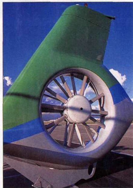
The EC130's Fenestron has unequally spaced blades, the key, says Eurocopter, to lower noise and vibration levels
