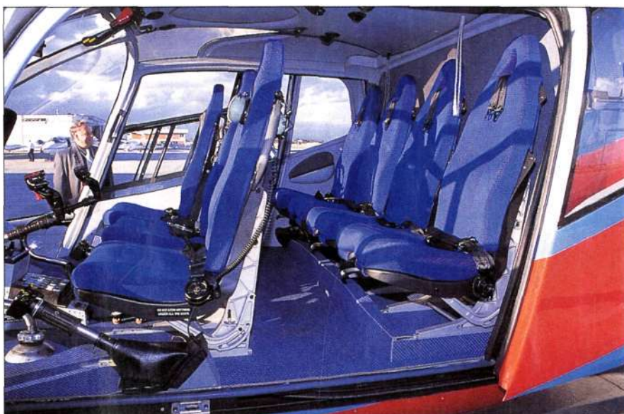
The rear four seats are elevated to increase passenger external visibility
