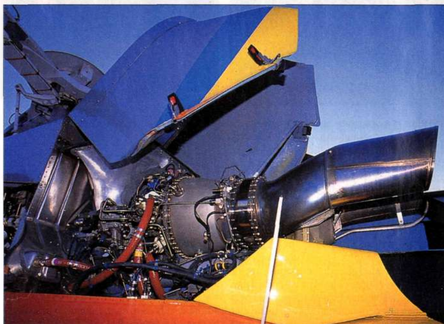
(Top) The EC130 has excellent rotor characteristics; (above and middle left) the Turboméca Arriel 2B1 engine has two FADECs; (middle right) the baggage compartment has more space than its competitors
