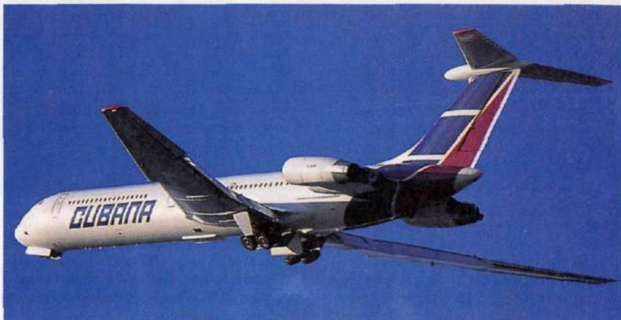
A hushkit and new operating procedures have been developed to reduce the noise levels of the Il-62
