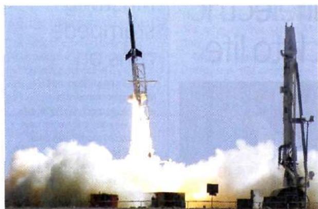
July test demonstrated successful supersonic combustion
