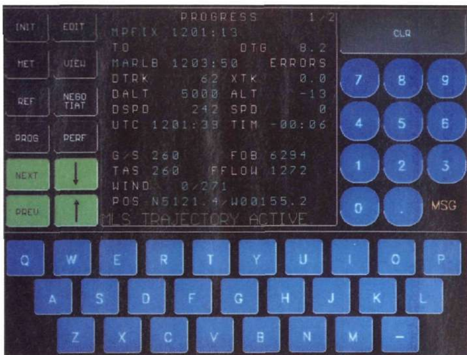
The experimental CDU's touch-screen may be replaced because of its sensitivity
