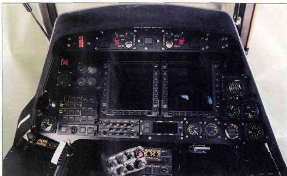
The pleasantly uncomplicated cockpit is dominated by two multi-function displays
