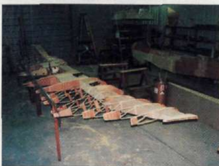
All-wooden construction makes Robin's DR400 and DR500 unique in the touring market
