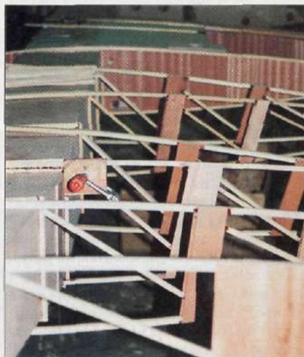
All-wooden construction makes Robin's DR400 and DR500 unique in the touring market
