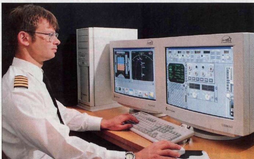
TTS' Boeing 737NG desktop flight management system trainer is an example of product innovation
