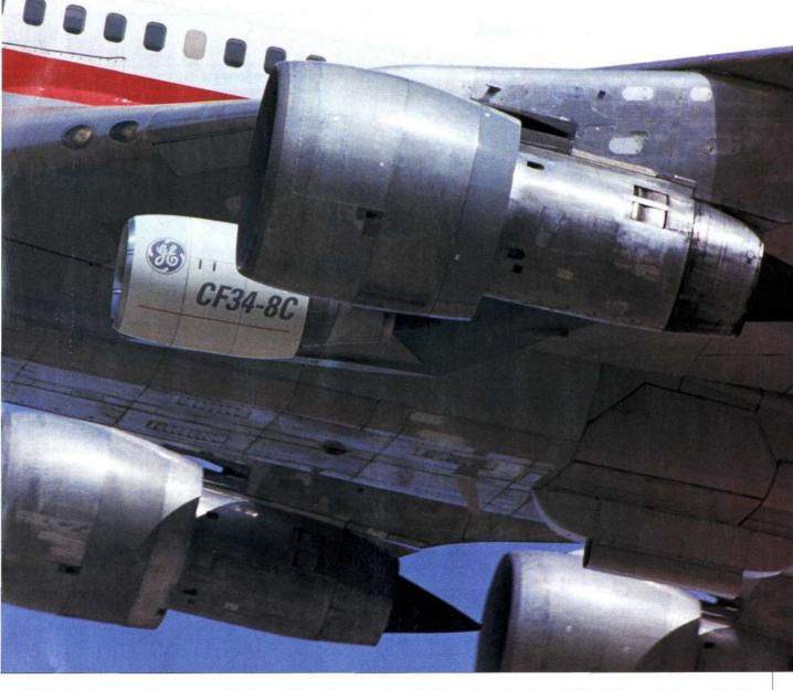
blades also feature cooling to cope with the higher operating temperatures of the larger engine. It also has boltless blade retainers, derived from similar technology adopted for the growth CF6 models, which increase component life. The low pressure (LP) turbine is similar to the -3A/3B1 rotor structure, but is otherwise different on the -8C1. The turbine consists of four stages, each designed using
