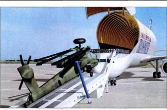
Airbus' on-board cargo lifter makes the Beluga self-loading
