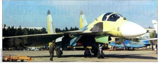
The Su-33KUB could be the first in a line of two-seat naval Flanker derivatives
