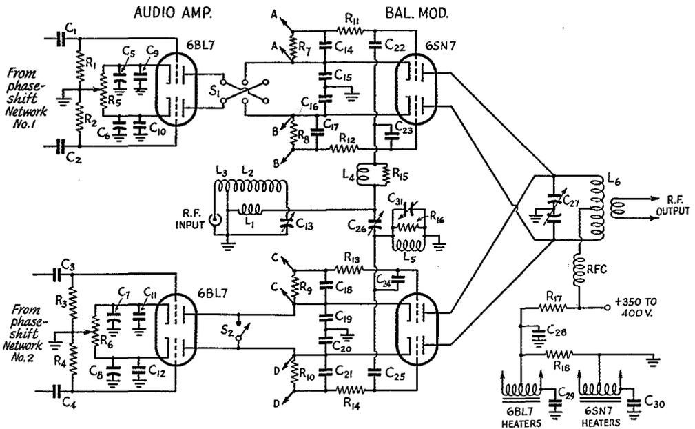
Fig. 2 — The series balanced-modulator circuit of W8DLI eliminates the need for audio coupling transformers. By-pass condensers and metering circuits make it look more complicated than it actually is.
