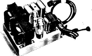
TYPE APS-50 — delivers 425V at 275 ma., and 6.3V and 4 amps. May be mounted on rack panel. For 110V AC, 50-60 cycles. Hi-lo switch on high voltage. Two 5U4G rectifiers. 11 x 6 7/8 x 8 3/4". 27 lbs.
