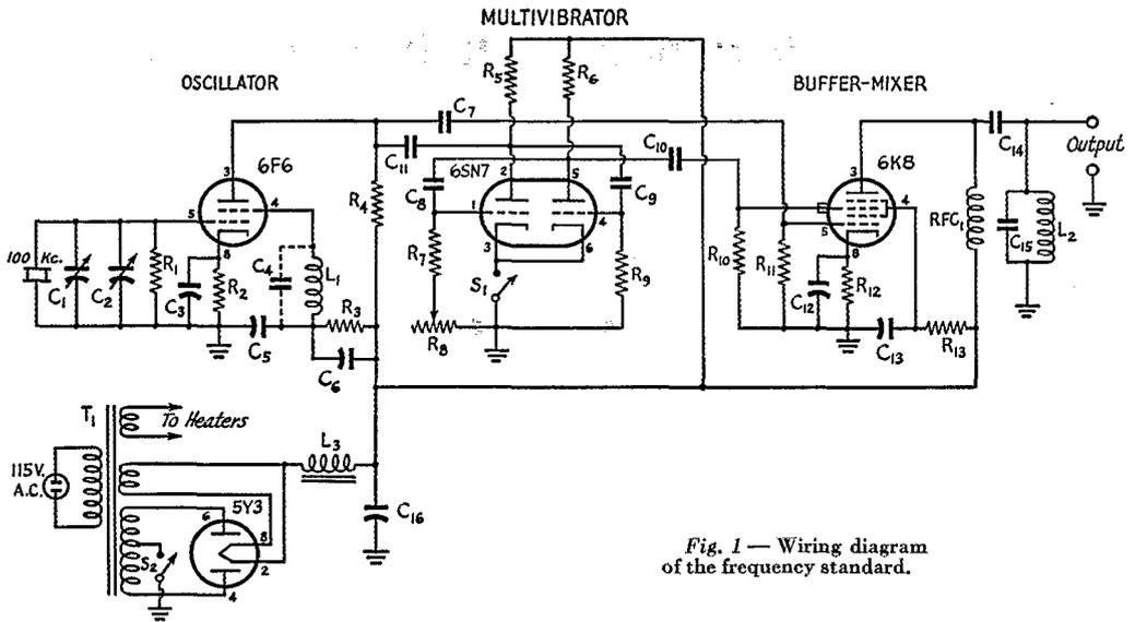
Fig. 1 — Wiring diagram of the frequency standard.
