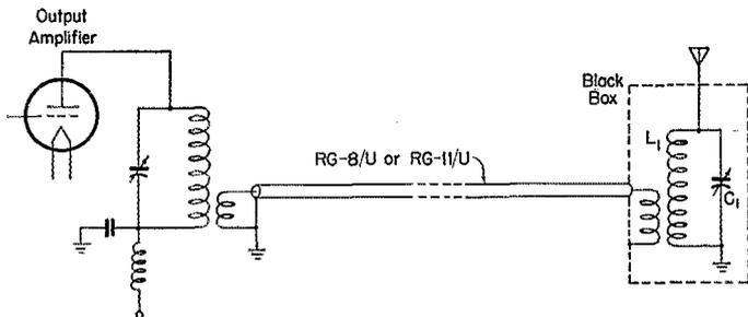
Fig. 1 — The "black box" antenna tuner is coupled to the output amplifier through a length of coaxial line.  $L_1$  and  $C_1$  should resonate to the operating frequency — when the antenna is connected it will require retuning unless the antenna is a quarter or half wavelength long. As described by W4SZU, the black box is very useful in feeding random lengths of wire.
