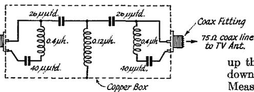
L<sub>1</sub> & L<sub>3</sub> = 40 turns C.T. of No. 30 enamel close-wound on 1/8" dia. knitting needle (plastic)
