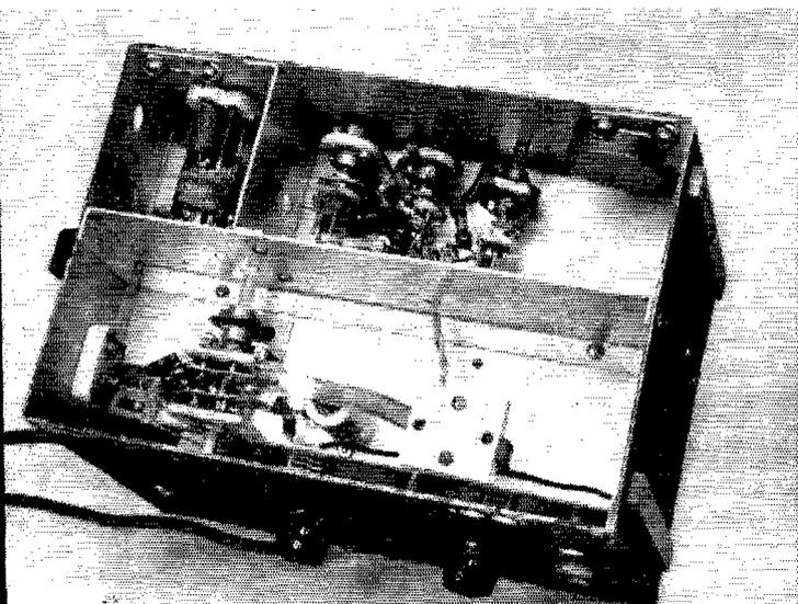
Looking into the bottom of the 432-Mc. converter, we see the r.f. amplifier components in the large compartment. The shielded tube is the 6AK5 i.f. amplifier. Oscillator and multiplier circuits occupy the two upper sections.
