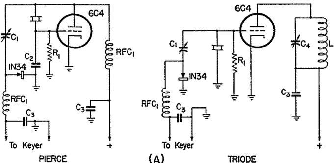
Fig. 3 — In these circuits a diode is used as a remotely-controlled relay. The remainder of the circuit of B is the same as Fig. 2.
