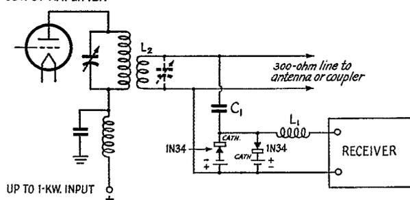
Fig. 1—The basic circuit for one-antenna break-in operation without a relay.  $C_1$  and  $L_1$  resonate near the amateur band being used. If the transmitter runs less than a kilowatt, the value of  $C_1$  can be increased and the value of  $L_1$  decreased accordingly.
