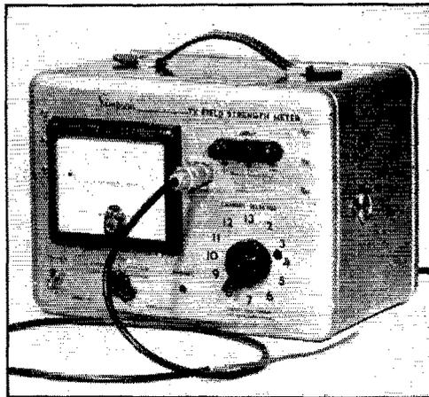
The modified TV field strength meter used for checking harmonic radiation. A coax fitting is installed for use with RG-59/U and a hole is drilled in the panel to permit retuning the oscillator beyond the fine-tuning range provided.
