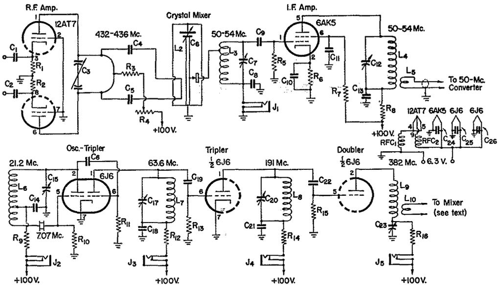
Fig. 1 — Schematic diagram of the 432-Mc. converter built by WIHDF.
