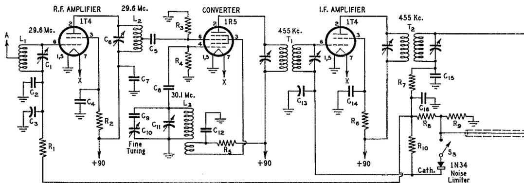
Fig. 1 — Wiring diagram of the 10-meter battery-powered station.
