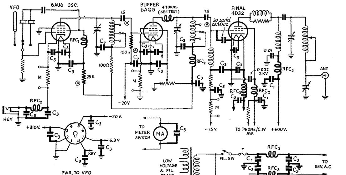
Fig. 2 — Essential circuits of the Viking, showing modifications in heavy lines. Changes marked with the symbol A in a circle were not made for TVI reduction, but to increase the final grid current on 10 meters. The following parts are required:
