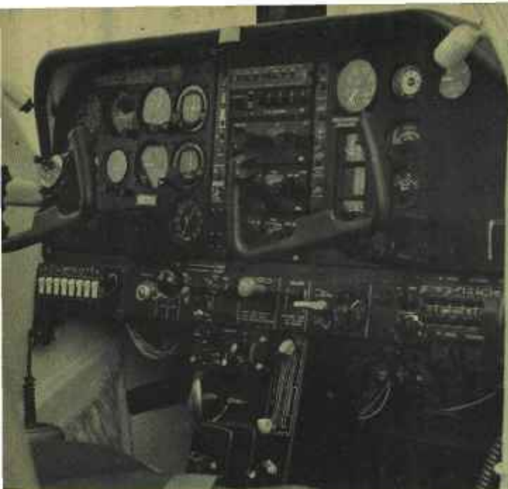
The extremely well-equipped cockpit of the Diplomat demonstrator. The autopilot is mounted beneath the throttle and propeller control
