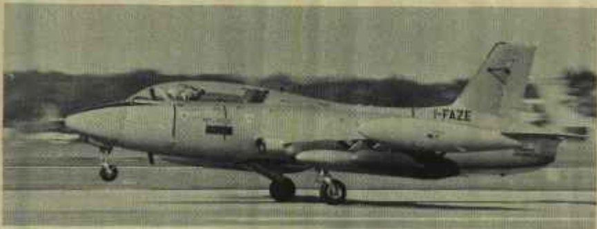
Three of the overseas aircraft sponsored by Rolls-Royce. Viper-driven are the Macchi MB.326G (left) and the Soko Galeb in the foreground (below), while the Grumman Gulfstream II, behind, uses Speys to achieve peak performance in the executive jet category
