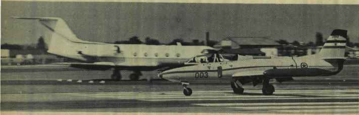
Three of the overseas aircraft sponsored by Rolls-Royce. Viper-driven are the Macchi MB.326G (left) and the Soko Galeb in the foreground (below), while the Grumman Gulfstream II, behind, uses Speys to achieve peak performance in the executive jet category
