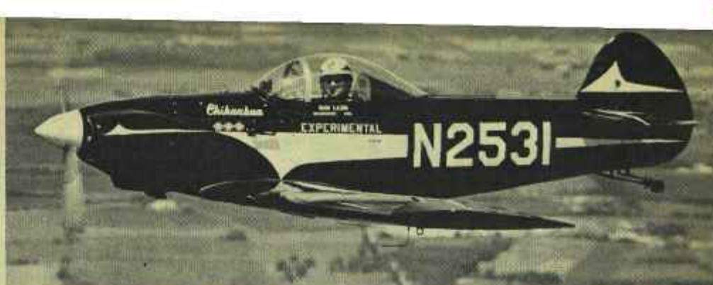
Above, Robert Ladd has made further modifications to his Taylor Monoplane, fitting it with retractable main gear using go-kart wheels, tyres and brakes. Power for Monoplane is a 42 h.p., 1,500cc VW and the aircraft received the award for the outstanding contribution to low cost sport flying
