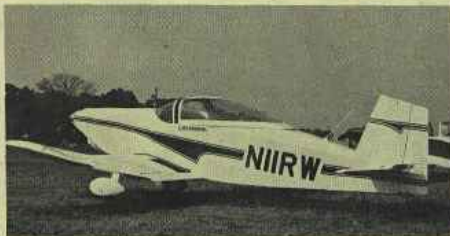
Right, The award for the best all-metal aircraft went to Richard Walen, who built this Standard T-18. The aircraft has Alumigrip paint and a hand-carved, leather interior with rolled and pleated seats. It has a 135 h.p. Lycoming which gives it a cruise speed of 170 m.p.h., 270 k.p.h. Bottom right, Wiley Post and Charles Lindbergh were perpetuated by these two near originals based at Oshkosh. Lockheed Vega, "Winnie Mae" (right) gained Grand Champion antique award for second year running. Left, the Ryan Monoplane
