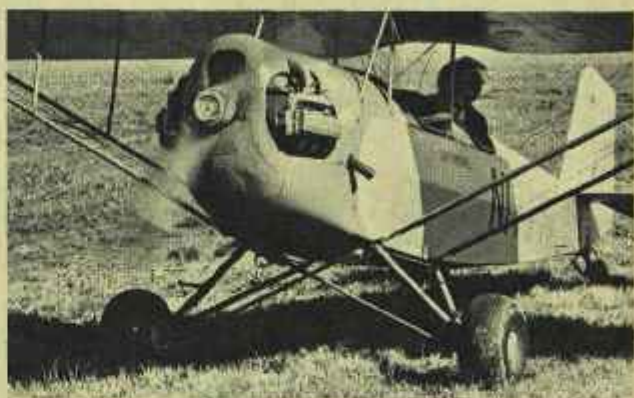
Above, a 1966 70 h.p. Corvair Corsa car engine is fitted in this two seat Pietenpot Aircamper built by Byron Petersen. Construction is all wood. It was built in Hawaii and later shipped to Torrance, California. It was flown the 2,300 miles, 3,700 km from there to Oshkosh
