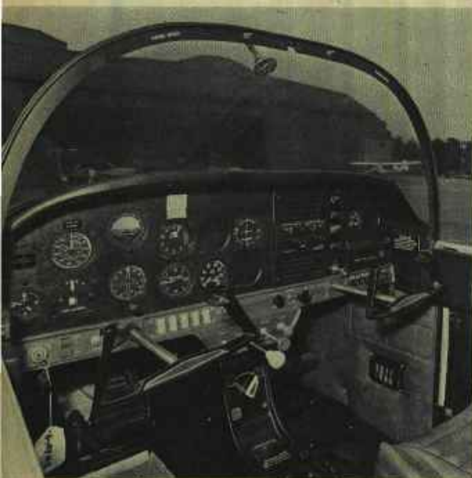
Above, the full panel and the radio are standard fittings in the Yankee as delivered in Britain. The unusual fuel gauge can be seen on the right-hand cockpit side
