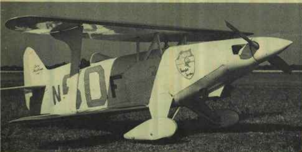
Left and above, a Knight Twister Imperial with a racing aerofoil developed by Twister designer V. Payne and built by flying instructor, D. Fairbanks. Engine is a 135 h.p. Lycoming O-290 D-2. Below left, a Jeanie's Teenie Mark 2 built by Cal Parker. This version has a less angular layout than earlier ones. Construction is all aluminium with VW power. Below, Sam Burgess built this Jungmeister in Honolulu
