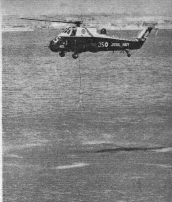
"Engadine" helidunk: a Wessex HAS.3 lowers the body of its Mk 195 sonar. Datum hovering height during the dunking phase is 40ft with an automatic "inching" facility to maintain at least 25ft separation between the aircraft and the wave crests. The Wessex 3 is claimed to have detection capabilities equivalent to those of a frigate
