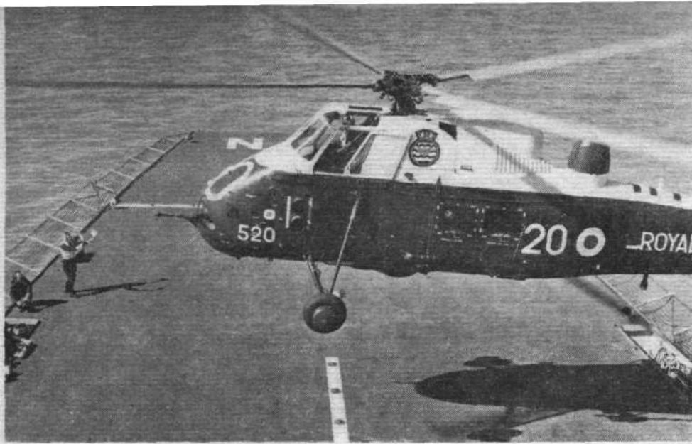
A 737 Sqn Wessex HAS.3 makes a cross-deck landing for a running turnround on the two-spot flight deck of the new RFA "Engadine," the first purpose-built helicopter support ship in Royal Navy service
