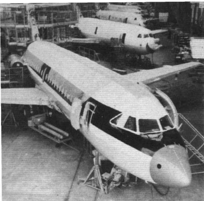
BAC's Hurn factory has built more turbine-engined short-haul aircraft than any other in the world. There are two lines of One-Elevens—400 series (left) and 500 series (right)
