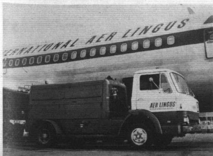
A useful source of hot air for defrosting aircraft parked in the open is a vehicle such as Atlas Copco's Air Partner ground air starter
