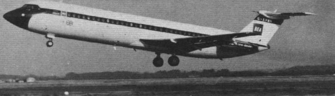
Super One-Eleven attitude after lift off is normally limited to less than 20° for passenger comfort, though the aircraft climbs well at even lower speeds a nearly flat attitude is adopted prior to the landing flare
