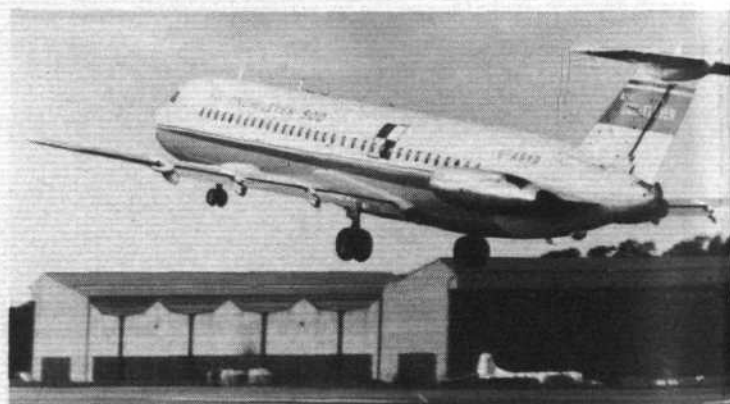
BAC actually stretched the original 400-series development aircraft (G-ASYD) to make it an aerodynamic prototype for the 500. It is seen here taking off from the test airfield at Wisley
