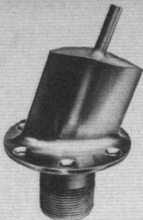
Protruding only 2½ in from the surface on which it is mounted, the Rosemount ice detector head depends on change of resonant frequency caused by ice build-up
