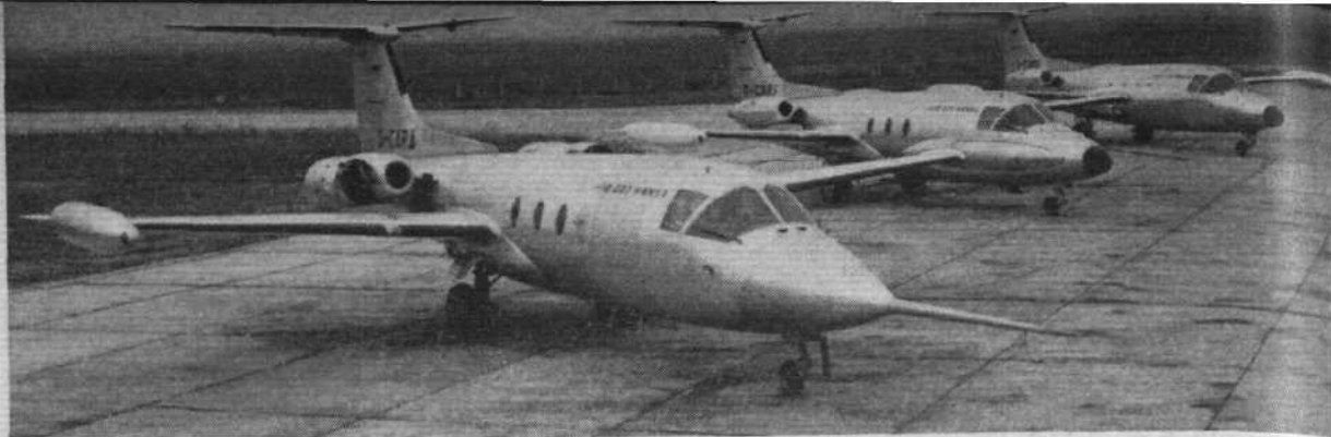
Three production-standard HFB 320 Hansa business jets on the flight line at the Torrejon, airfield, near Madrid where certification flying is now nearing completion. Four HFB 320s are now flying; recent external configuration changes include the fitting of boundary-layer control fences on the wing and tailplane
