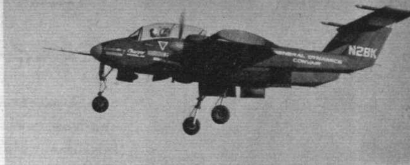
The Charger gets away from Lindbergh Field, San Diego, with take-off flap and gear extended
