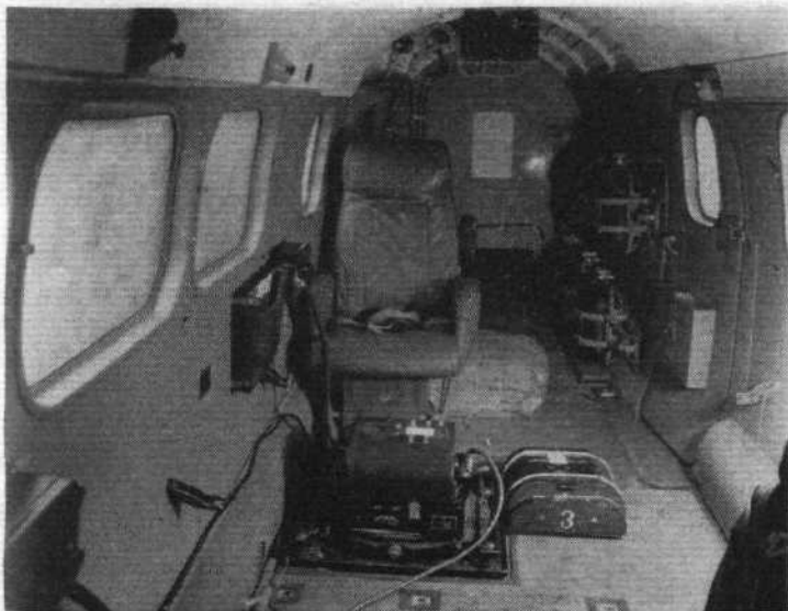
Williamson F.49 6.3in camera in a Dove survey aircraft
