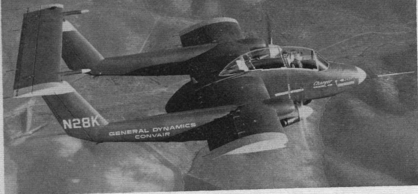
Still civil registered, Convair's Charger flies in clean configuration during its first 27hr flight test programme
