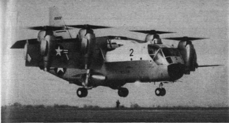
First hovering flight, with flaps not deflected, was made at Dallas on December 29 by the Vought-Hiller-Ryan XC-142A. Following the first flight with 10° wing tilt, several other flights were made with other deflection angles before the present VTOL programme started
