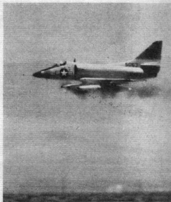
Hughes Aircraft has received a $9,568,350 order for Hipeg rapid-firing 20mm gun pods from the US Navy. The Douglas A-4 Skyhawk above is firing three Hipeg pods with a combined output of more than 12,000 rounds per minute
