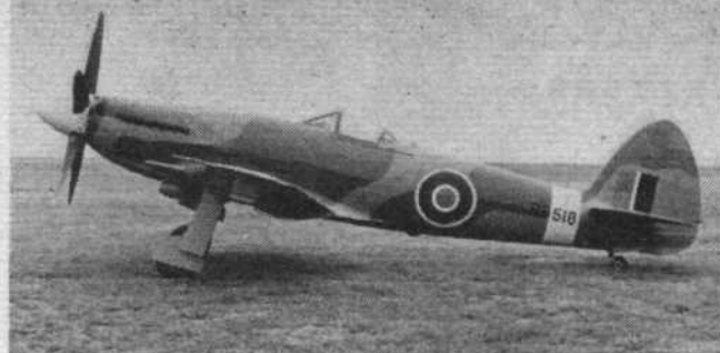
The Vickers-Supermarine Spiteful (see letter from Mr T. Connaughton) was a post-war descendant of the Spitfire, with straight-tapered, square-tipped wings and a deeper fuselage. This is the Rolls-Royce Griffon-powered F.16 Spiteful which in 1947 attained a speed of 494 m.p.h.
