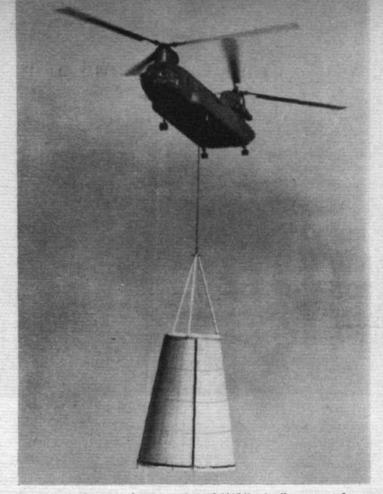
This  $2\frac{1}{2}$ -ton dummy adapter section of NASA's Apollo spacecraft was delivered from North American Aviation's plant at Tulsa, Oaklahoma, to Cape Kennedy, a distance of 1,000 miles, by US Army Chinook helicopter in 16 flying hours. The trip was made in five legs with two over-night stops, cruising at 2,000ft and averaging 90 m.p.h.
