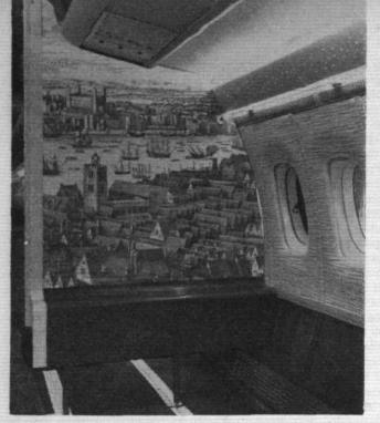
An effective Formica "London 1647" black-and-white impression covers the transverse bulkheads of the passenger cabin of BOAC's Super VC10. The prefabricated sidewall trim, with integral airconditioning and cornice lighting, is also seen, together with the "floating" overhead rack and the recessed and movable passenger service panels
