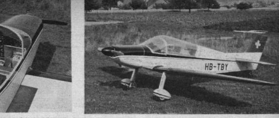
Now being produced by Uetz at Fehraltorf, Switzerland, is the U4M Pelikan, which received its Swiss C of A last June. Salient details are: span, 31ft 7in; length, 24ft 7in; wing area, 142 sq ft; empty weight, 1,132lb; gross weight, 2,200lb; engine, 150 h.p. Lycoming 0-320; max speed, 135 m.p.h.; cruising speed, 123 m.p.h.; stalling speed, 41 m.p.h.; rate of climb, 700ft/min; take-off run, 740ft; service ceiling, 14,600ft; range, 620 miles; price in Switzerland, SFr 45,000 (about £3,720)
