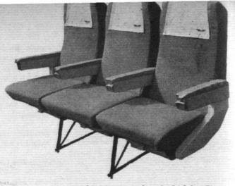
Fig 3 Typical tourist-class seat as used on the BAC One-Eleven
