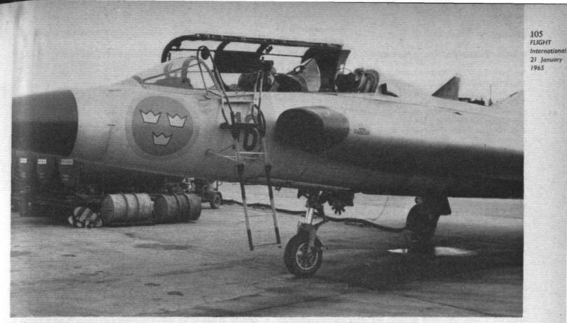
The Sk35C trainer cockpit shows the distinctively sharply raked ejection seats, inner blast screen recessed to take the periscope mounted in the black centre canopy panel, the access ladder and the extended ram-air turbine aft of the nosewheel leg. The Sk35C carries neither radar nor missiles
