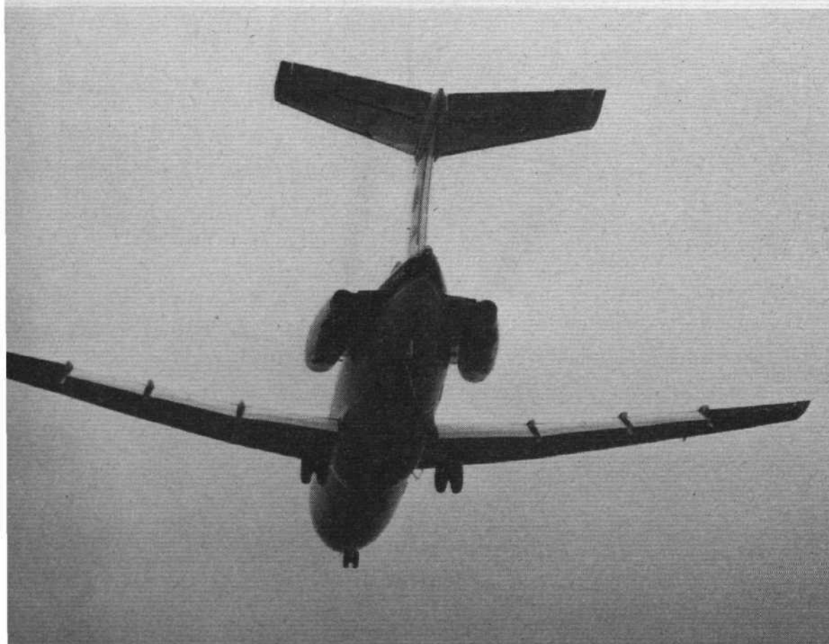
G-ASJC (above) was the aircraft mainly responsible for a stalling programme of unprecedented severity and thoroughness. The new powered elevators were fitted first to G-ASJD (left)
