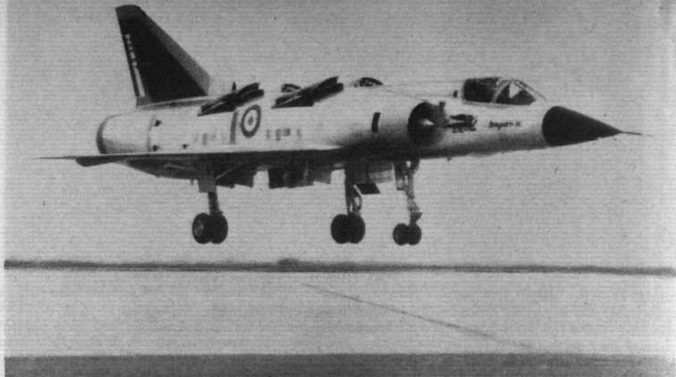
IIIV in the Z Axis: René Bigand, Dassault chief test pilot, making the first vertical take-off in the Dassault Mirage IIIV at Melun-Villaroche on February 12, also marks the first lift-off of the Rolls-Royce RB.162 engine. Propulsion engine is here an early SNECMA TF-104, to be replaced soon by the first TF-106 recently delivered to Melun. The definitive TF-306 will be fitted late this year for supersonic flying. Both the Mirage IIIV and Balzac may be at the Paris Show. The IIIV will become the third VTOL to exceed Mach 1, but the first operational VTOL with level supersonic performance. Its gross weight is approximately 26,500lb. Noteworthy are the efflux deflector doors for ground-running and short take-offs.
