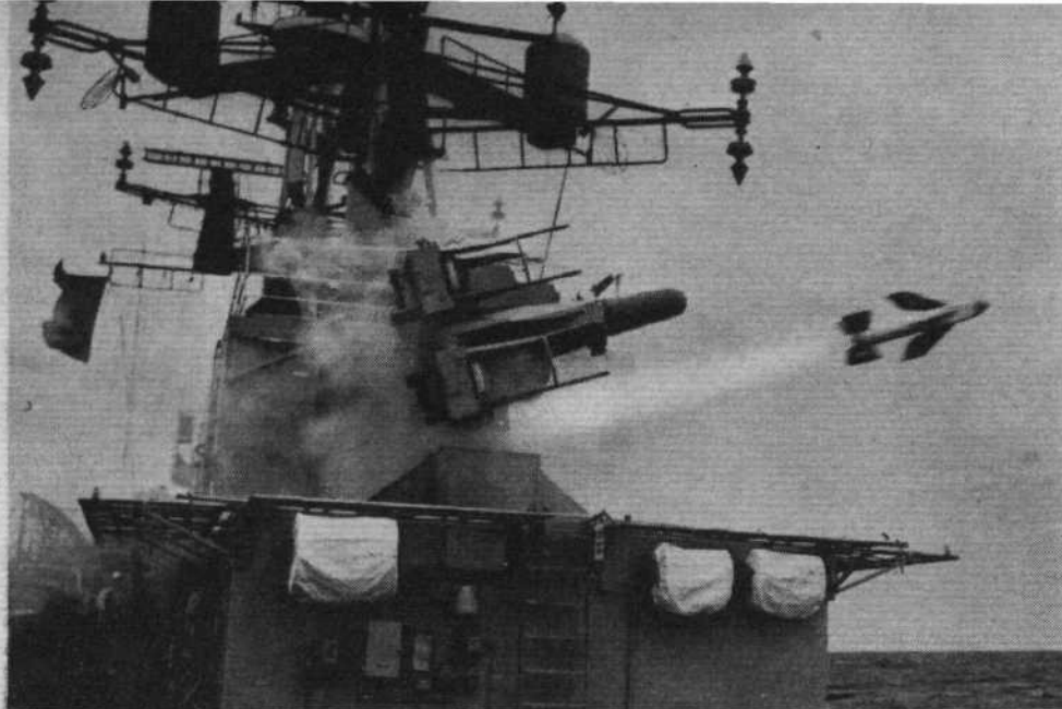
One of seven Short Seacat missiles departs from HMAS "Yarra," the RAN's third missile frigate, to intercept a drone aircraft launched from the same ship. The firings were made off the coast of New South Wales to prove the installation
