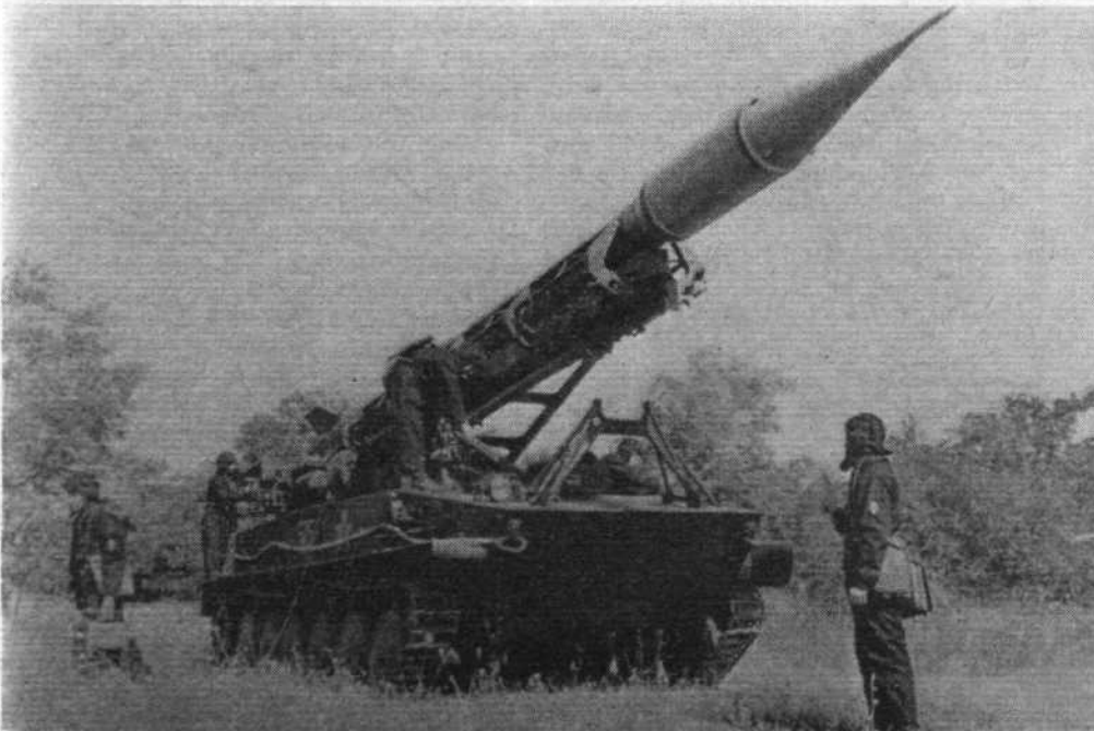
Russian troops prepare to launch a Frog tactical missile. One man is folding down the ramp support stay while another walks away unreeling the firing cable. Altogether six men are visible
