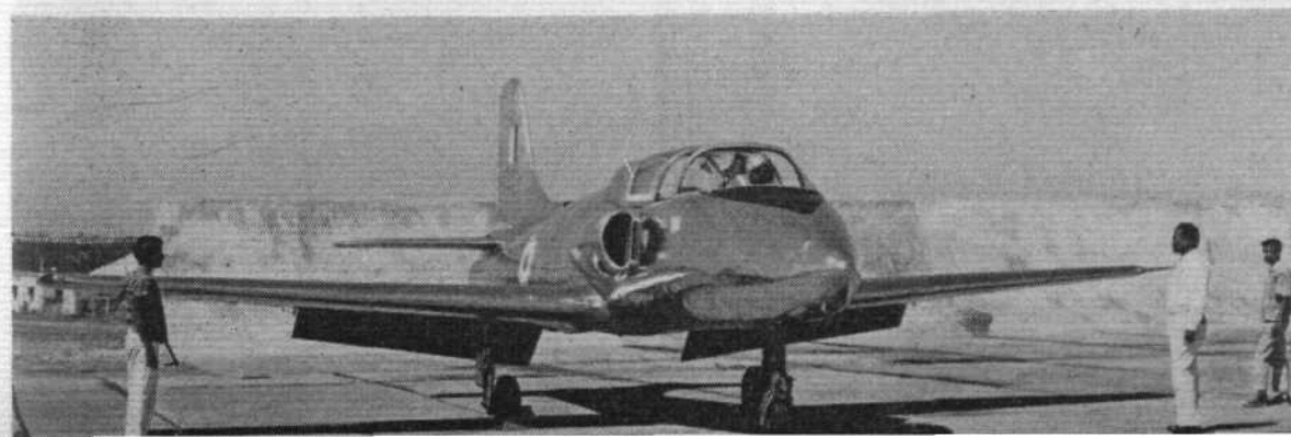
Design of the intakes for the Viper 11 engine reconciles adequate performance with the benefit of a simple wing-root structure
