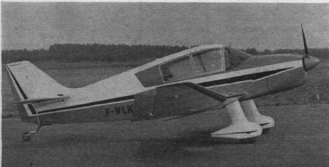
The 140 h.p. four-seat Centre Est DR 250 Quadriplace ("New Jodel From Dijon," above) promises to be a fast and efficient newcomer from France. An interim development aircraft called the DR 200 has been flying for some months and is externally similar to the DR 250 but is powered by a 105 h.p. Potez engine
