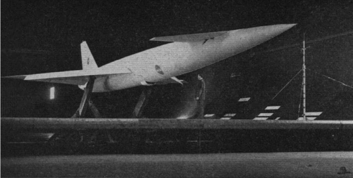
This one-third scale model of a generalized design for a Mach 3 transport is used in the 40ft x 80ft wind tunnel at Ames Research Center to obtain basic low-speed information. The canard model's delta wing is fitted with large flaps on both leading and trailing edges to increase lift at low speeds. Beneath the model but above the floor is a ground plane used to study ground-cushion effects
