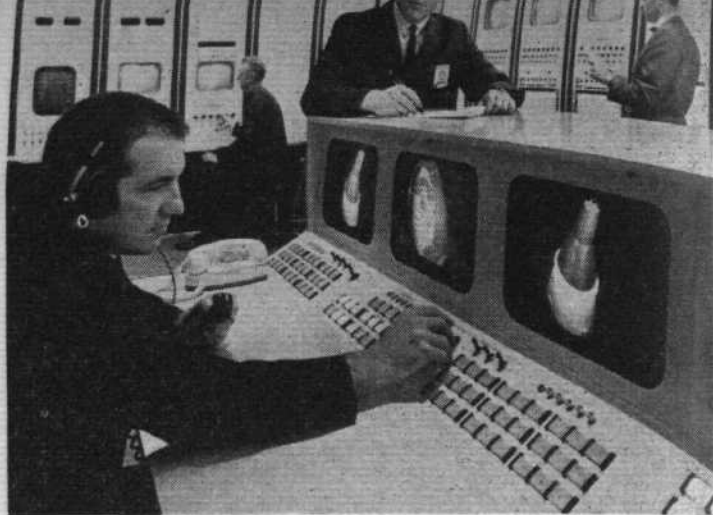
An integrated manned space systems simulator is being installed at the Convair division of General Dynamics, San Diego. When the unit is operational, a test conductor will be able to monitor from this control console a simulated mission being flown in a spacecraft in an adjoining room. Models in the closed-circuit television system are computer-driven to display the astronauts' view: engineers will use the simulator to study design requirements for a manned orbital laboratory and other spacecraft
