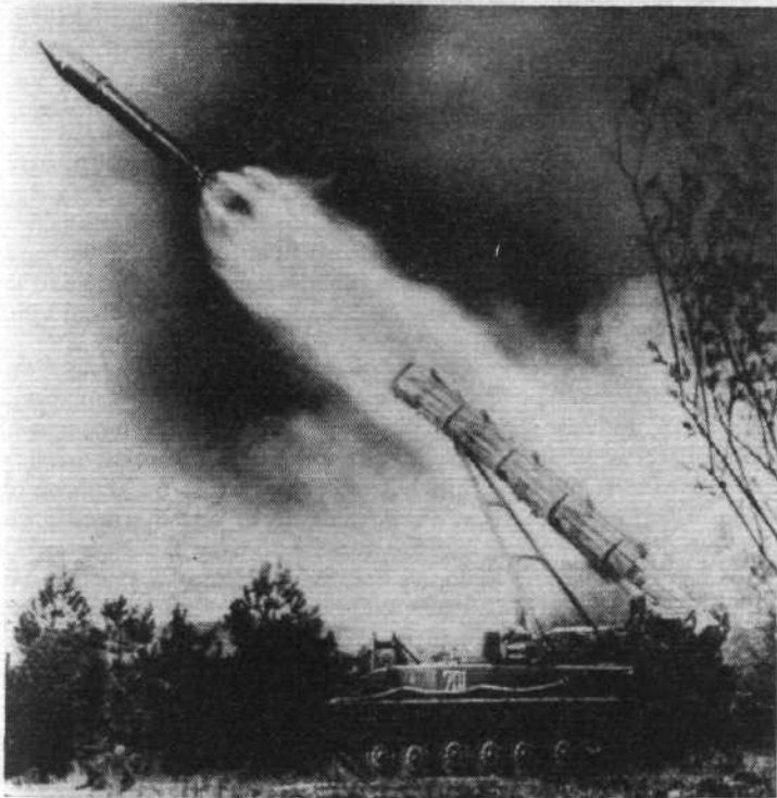
Russian troops prepare to launch a Frog tactical missile. One man is folding down the ramp support stay while another walks away unreeling the firing cable. Altogether six men are visible
