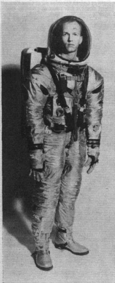
The astronaut's space-suit developed for NASA's Apollo programme and described on this page, worn here by a Hamilton Standard engineer, over whose right shoulder can be seen the portable life-support back-pack
