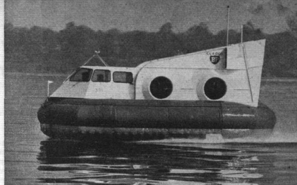
The prototype CC-4, built for HDL, is now engaged in skirt development trials. The second prototype, now taking shape at Bembridge, incorporates substantial changes, though it retains the integrated lift and low-velocity jet propulsion system and the R-R LV-8 powerplant. Plans are being made for its production in quantity
