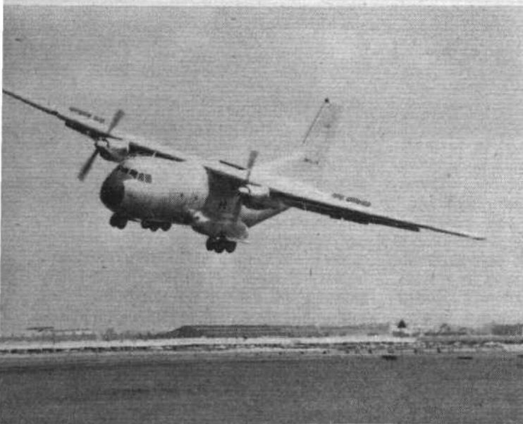
Three Franco-German Transall C-160s took part in the flying show. Airbrakes are extended for this short-field approach
