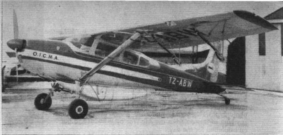
Bournair, the Hurn Airport Cessna dealers, recently supplied a Cessna Skywagon to the Organisation Internationale Contra le Criquet Magrateur African in Mali. Bournair fitted the aircraft with a 160gal Sorensen tank and also the Britten-Norman Micronair spray gear
