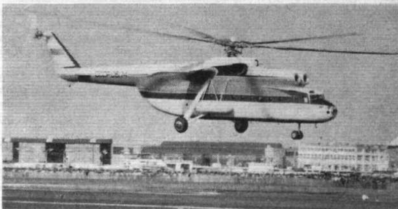
With short wings partially unloading the rotor in cruising flight, the Mi-6 transport helicopter—the world's largest—was a stately sight in flight. The powerplant/transmission/rotor combination appears to be used virtually unchanged for the Mi-10 flying crane
