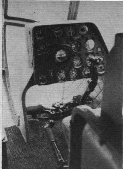
The flight deck of the Mi-8 is remarkably roomy and well windowed by Mi-6 standards. The two dials at top right serve the astro-compass system
