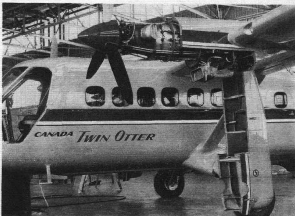
Right, the port Pratt & Whitney PT6A-20 turbine of the DHC Twin Otter with its top cowl removed and its lower cowl hinged down. The Twin Otter has two crew doors and two cabin-entry doors—one, on the port side, a double door, which is shown open in the picture below. It measures 46in by 45in
