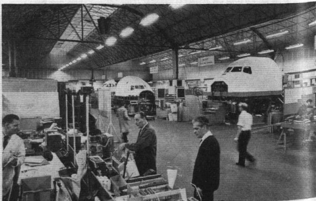
Simulators for Air Canada's DC-9 and Trans-Australia Airlines' Boeing 727 fleets are to be seen in this picture of work in the Redifon shops at Crawley, Sussex. The most recent order has come from Lufthansa
