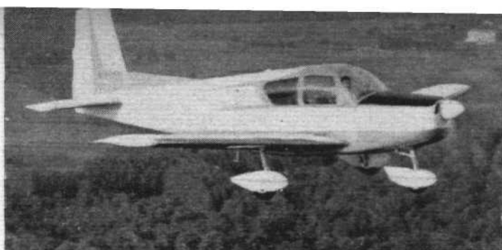
Italy's challenge to American domination of the European market for popular four-seaters is the SIAI-Marchetti S.205. Powered in initial form by a 180 h.p. Lycoming O-360, the spacious S.205 cruises at 134 m.p.h. on 75 per cent power
