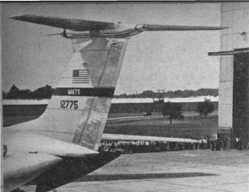
Fig 3 One of the largest examples of the "T-tail" yet built is that of the Lockheed C-141A StarLifter military transport, which rises almost 40ft from the ground
