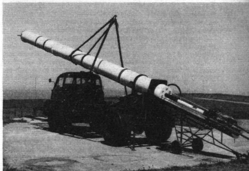
Operational firings of the 5in-diameter meteorological rocket were scheduled to begin as part of the IQSY programme from South Uist this week (see "Weather Rockets Launched"). Above, launching tube in launch position; above right, one of the proving firings; right, rocket (with boost motor attached) and launcher
