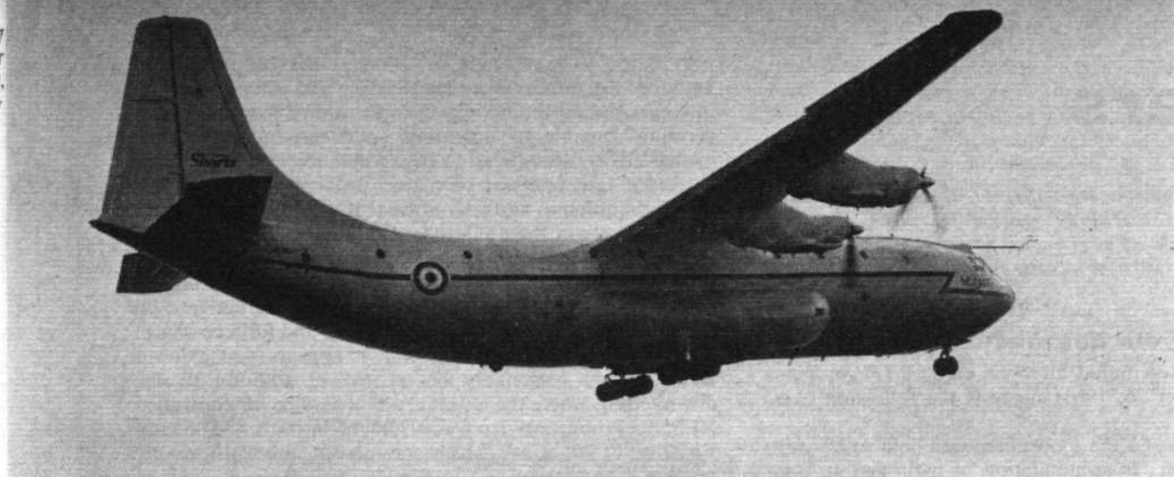
7 ... vortices stream again from the propellers as full power is called for the overshoot at altitude
