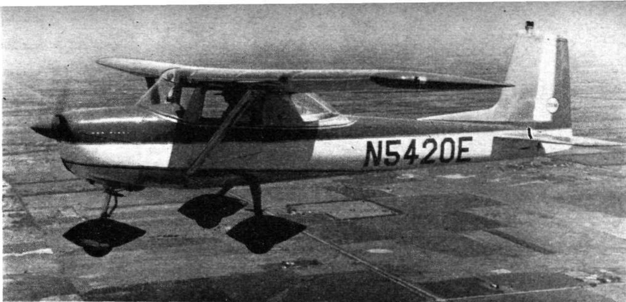
The 1964 version of the Cessna 150 incorporates the "omni-vision" rear canopy already featured on the larger Cessna types. Powered by a 100 h.p. Continental O-200A, the new 150 has an increase in gross weight from 1,500lb to 1,600lb. Price of the standard version is \$7,825
