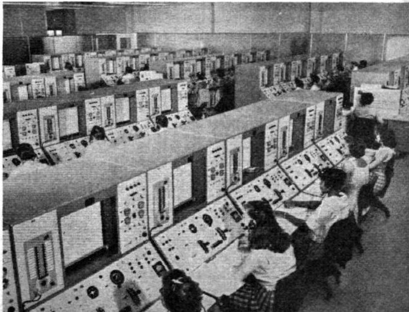
Some of the 60 single-track target generators and "pilots" in the FAA model B ATC simulator at Atlantic City
