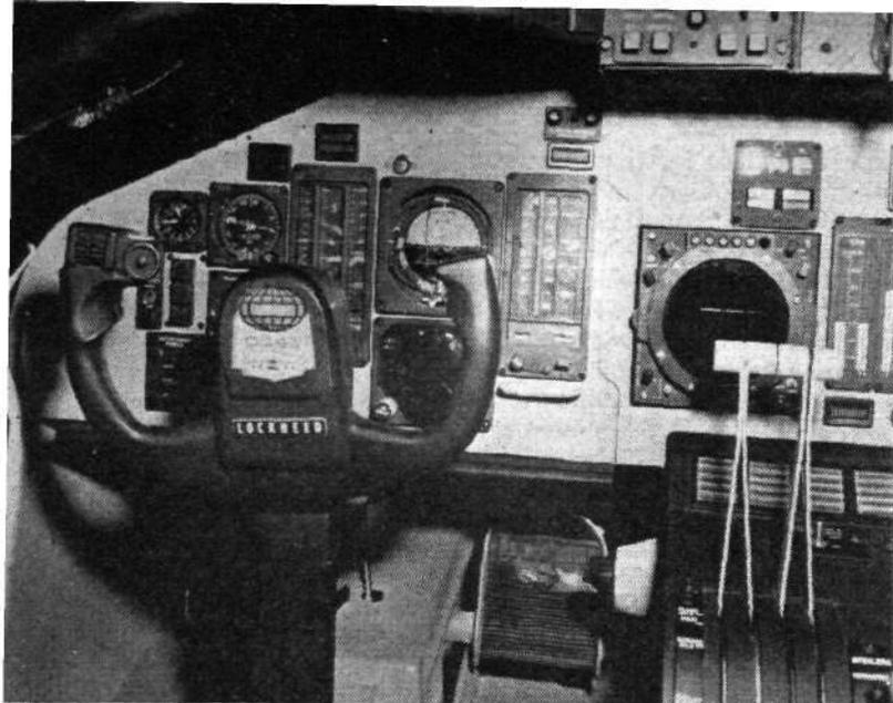
Captain's flight instrument panel for the Lockheed C-141 Starlifter, with dial flight directors and tape displays for speed and height values
