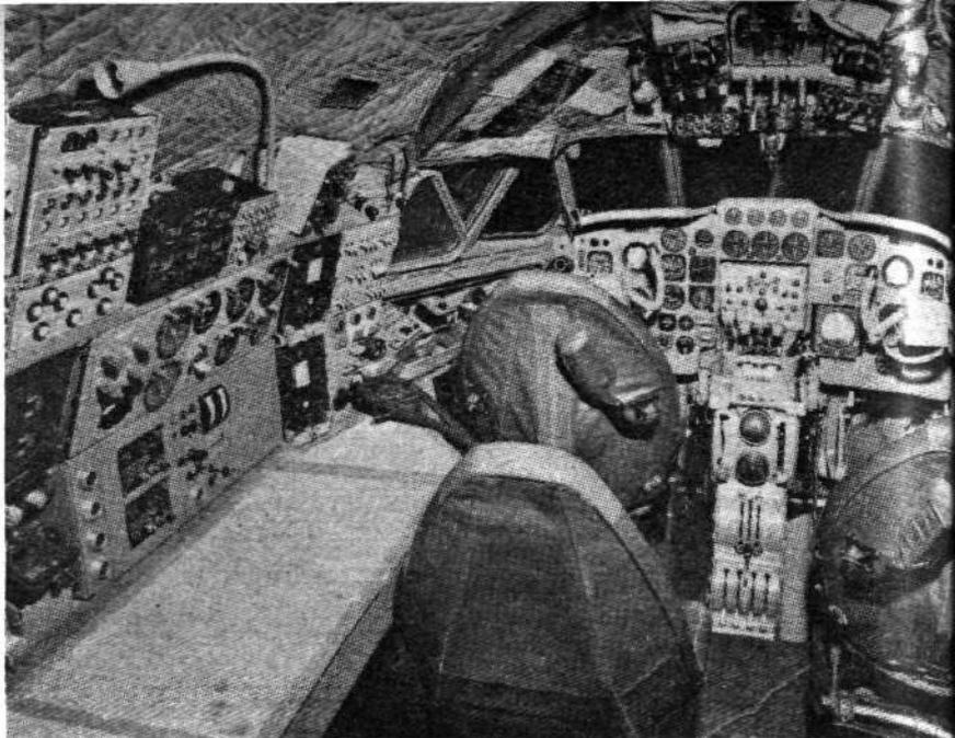
The BLEU Comet fitted for blind landing development with Smiths multiplex auto-pilot and instrumentation
