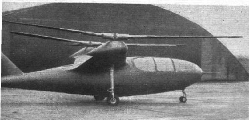
The Firth FH-1 helicopter referred to below; it utilized the fuselage of the Planet Satellite, an unorthodox low-wing monoplane of 1947-48.
