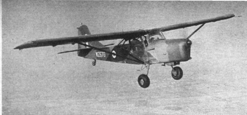
A.O.P. 9 IN SERVICE HANDS: Auster A.O.P. 9s (Cirrus Bombardier), of which this is one of the first aerial photographs, are now being delivered. Recently, 150 hours' of intensive trials were completed very satisfactorily, in the course of which 1,150 landings were made on rough strips. At one stage the aircraft was given a tremendous hammering in the form of intentional heavy landings, during which the Dowty landing gear proved its ability repeatedly to withstand between 3 and 4 g.
