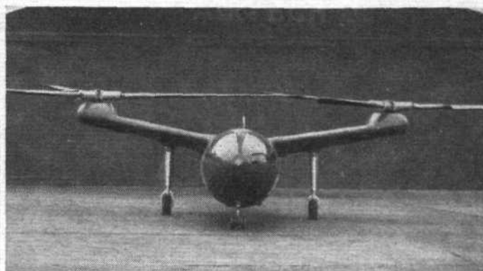
The Firth FH-1 helicopter referred to below; it utilized the fuselage of the Planet Satellite, an unorthodox low-wing monoplane of 1947-48.
