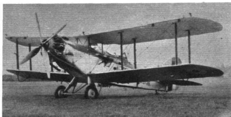
(Above) Long-fuselage Wapiti with experimental airscrew. (Right) Wapiti Ila seaplane (Bristol Jupiter VIII).
