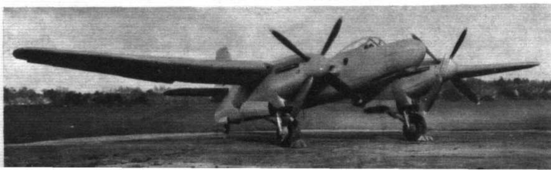
Welkin I (two Rolls-Royce Merlin 70 series). (Below) Welkin II (Rolls-Royce Merlin 76 and 77).
