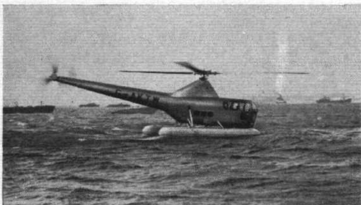
S-51, Series A, with pontoons (Alvis Leonides 521/1).
