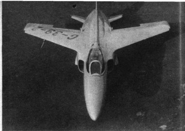
INSET AILERONS of the Folland Gnat, subject of "first flight" news (Col. 1), are well shown in this specially posed view, taken last week.
