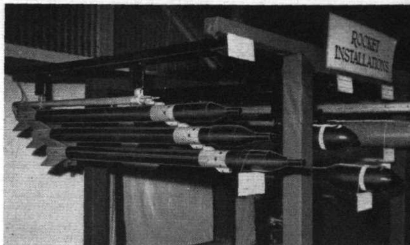
(Above) The 60 mm rockets, fin-stabilized and with offset thrust nozzles, and the finned 31 tube and plain seven-tube pods from which they have been fired experimentally. "Flight" photographs
