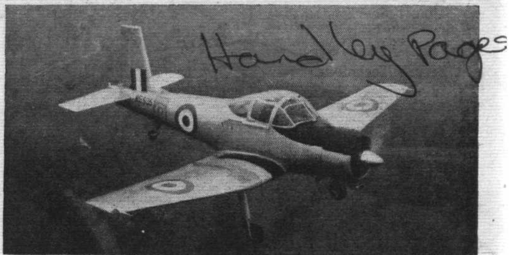
SIDE-BY-SIDE: These photographs, showing the Percival P.56 (upper picture) and Handley Page (Reading) H.P.R.2 display, comparatively, the external features of these Cheetah-powered basic trainer prototypes. Immediately apparent distinguishing features are the larger, curved-top fin of the Percival, and its straight leading-edge. The H.P.R.2's tailwheel-position (well forward) is another useful clue for the spotter. Both types may use the Alvis Leonides as an alternative power-plant. The Percival P.56 is now flying without the dorsal fin shown above.
