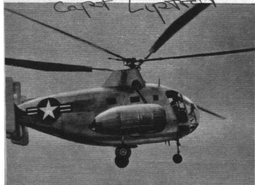
Twin-engined Kellett XR-10, with intermeshing rotors.
